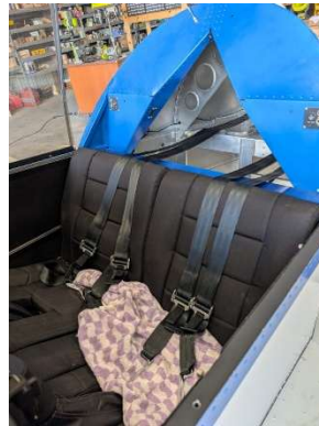
Seatbelt installation complete
