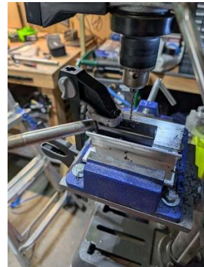
Pilot drilling new RH axle
