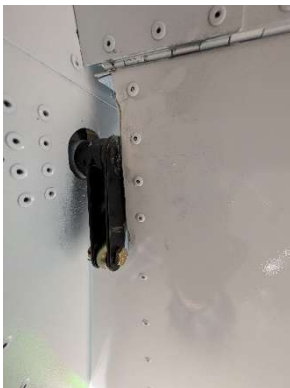
LH flap hardware installed
