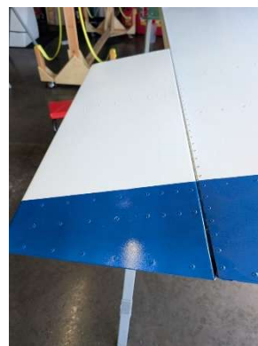
RH aileron installed with cotter pins
