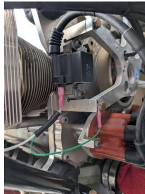
LH ignition coil wiring
