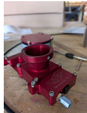
Air filter assembly mounting hole drilled and tapped
