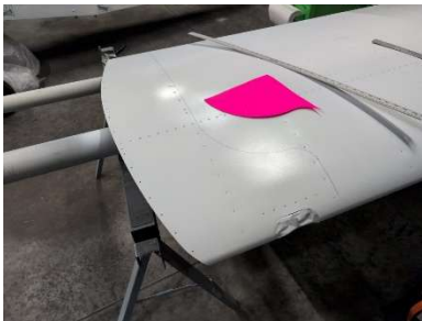
Laying out wingtip transition line on wing
