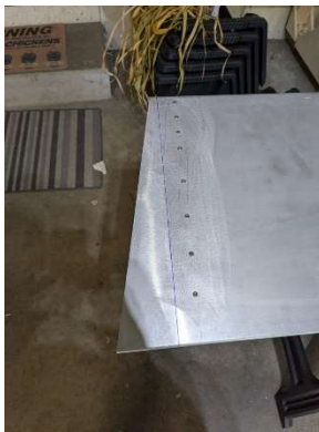
Inboard flap rib location marked
