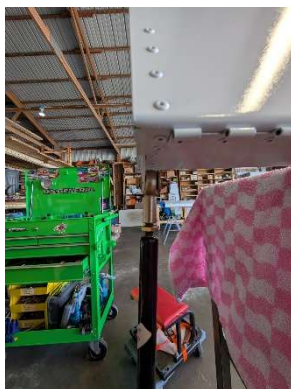
Pushrod assembly installed onto aileron
