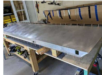
RH upper aft wing skin riveting complete
