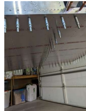
Aft tunnel web pilot drilled and clecoed to floor
