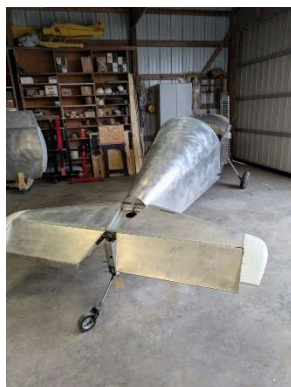
Horizontal stabilizer clamped into place and aligned via laser
