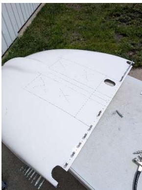
Exhaust tunnel layout marked
