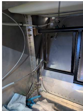
Fuel vent routed and connected inside cockpit
