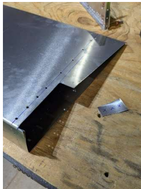
LH flap skin cut for pushrod clearance
