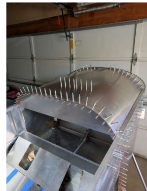
Instrument panel pilot drilled
