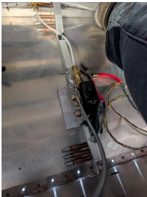
Parking brake cable installed and routed
