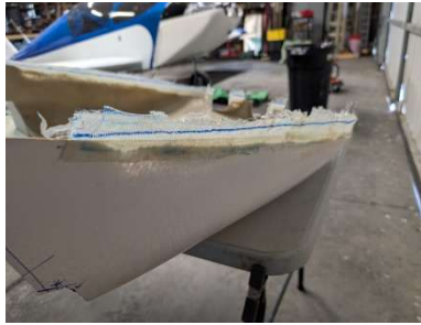
Rough trim line marked
