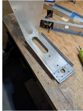
Riveted aft shear web assembly to aft bulkhead
