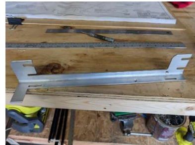
Canopy latch updrilled and countersunk
