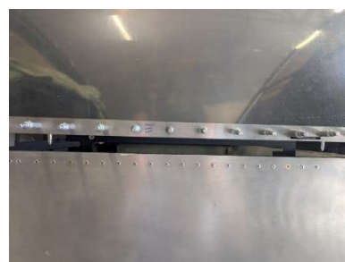
Upper canopy latch slots filed for tight fit but smooth operation
