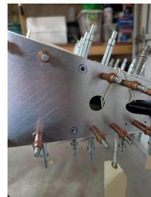
AN525 hardware holes updrilled
