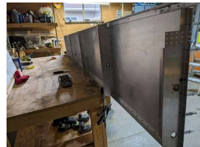
Bushings and grommets installed in vertical channels
