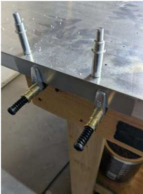
Skin simulator for lower longeron offset
