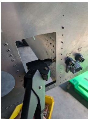
Flush riveting forward tunnel zee to wing mounts
