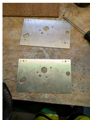
Brake fitting cutouts complete
