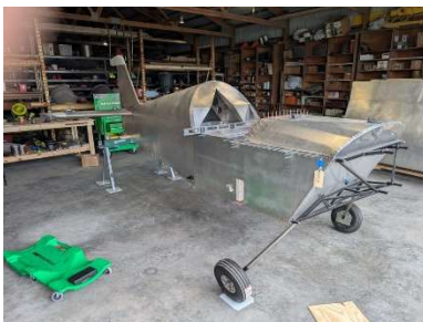
Fuselage leveling in progress
