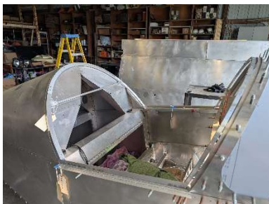
Canopy frame test fit into fuselage
