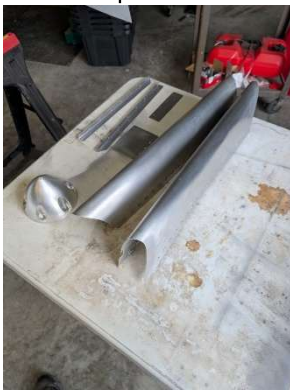
Aft fuselage floor prepped for paint
