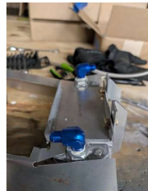
AN fittings installed in oil cooler
