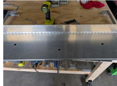
Rigging holes upsized
