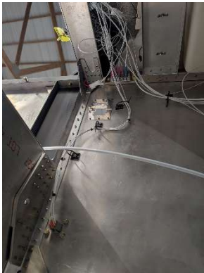
LH wing root wiring complete
