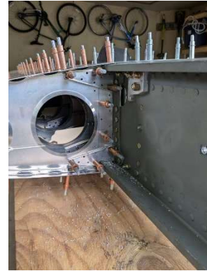
Forward root rib attach angle updrilled
