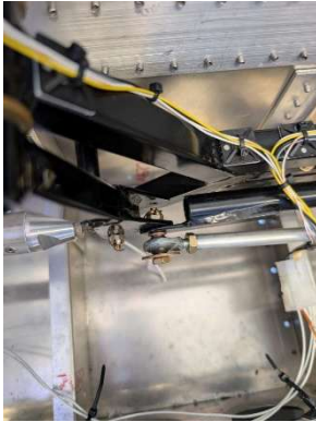
Servo push rod attached to control stick horn
