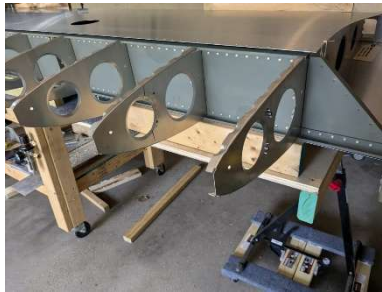
RH aft lower skin in progress
