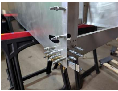
RH flap angle pilot drilled and clecoed
