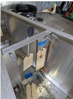
Pilot drilling F22-06 angle on #5 vertical channels
