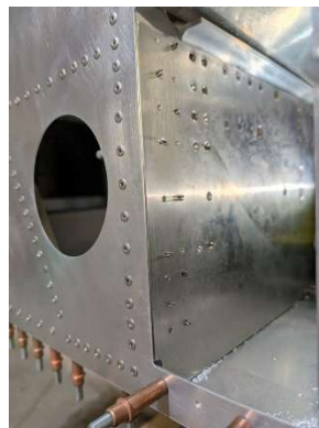
RH aft tunnel web updrilled
