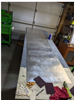
LH upper wing skin deburred and cleaned
