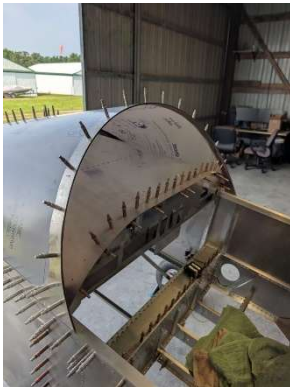
Rear edge of windshield pilot drilled
