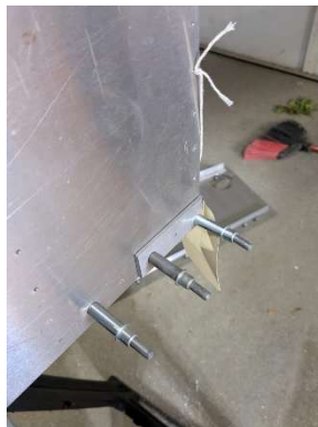
LH rudder stop mockup
