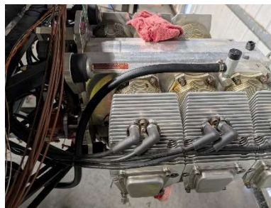
Oil separator line installed
