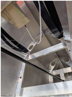
Shoulder harnesses bolted to seatbelt attach angles
