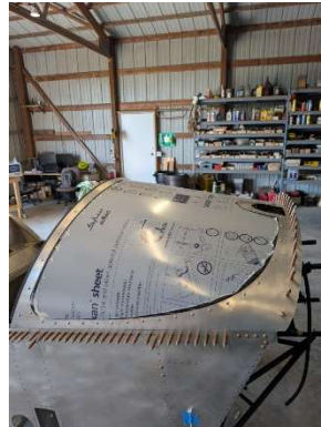
Screws installed in windshield and windshield bow
