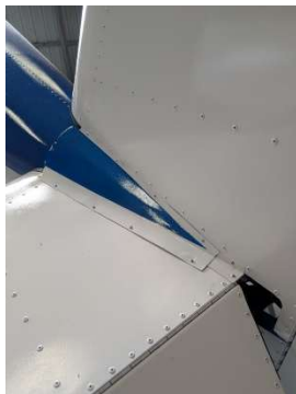
LH aft tail fairing angle painted and installed
