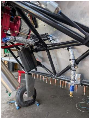
Fuel lines insulated
