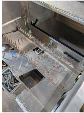
Rear seat pan updrilled
