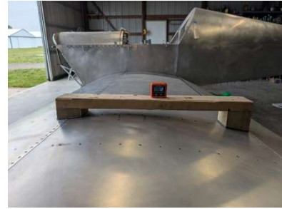
LH wing incidence angle being checked
