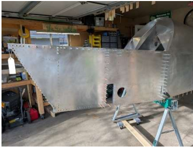
LH forward side panel clecoed into place
