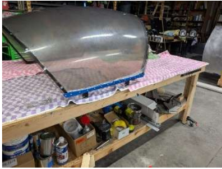
Canopy side trim installed
