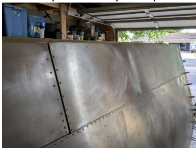
RH flap assembly installed
