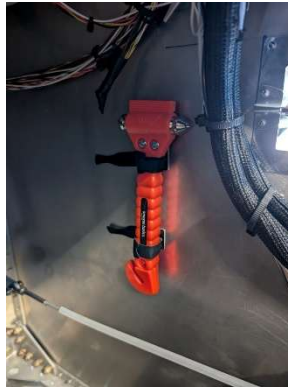
Crash hammer mounted on forward fuselage side panel
