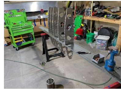
LH rib installation in progress
