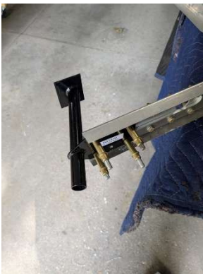
Updrilling tail wheel mount
