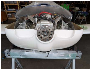
Lower cowl refit into place
