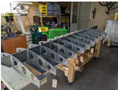
Ribs clecoed in place
