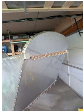
Upper firewall clecoed into place
