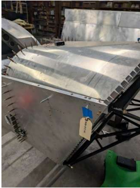
Windscreen bow clecoes and screws removed
