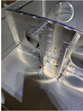
Aileron bellcrank support holes drilled
