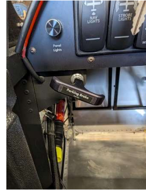
Parking brake decal applied
