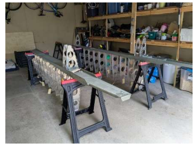
Forward ribs mocked up
