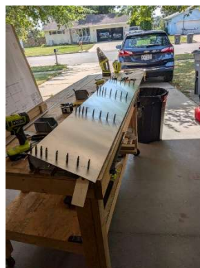
RH flap tip side pilot drilled
