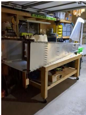
Testing tail fitment on aft fuselage section
