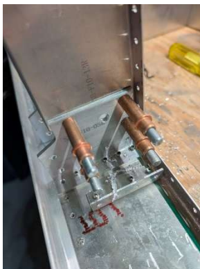
Seat belt mount holes transferred
