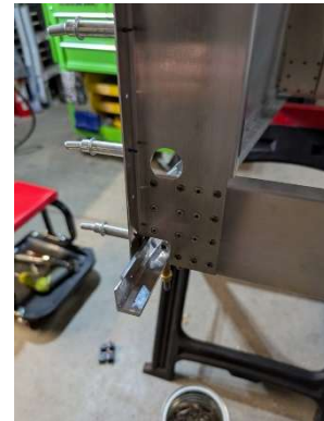
RH flap angle riveted
