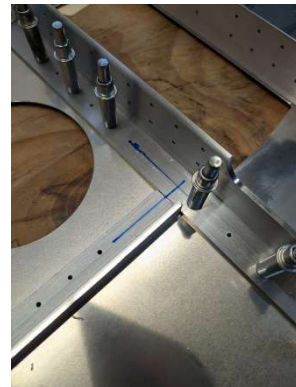
Centerlines marked for gussets
