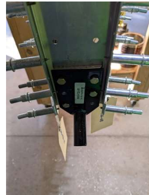
Aft tail wheel mount plate holes drilled through aft channel and lower support angle
