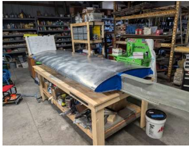
RH wing prepped for paint
