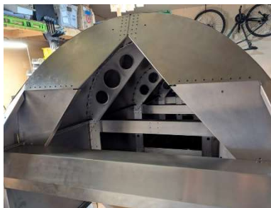
Lower #1 formers riveted to upper formers
