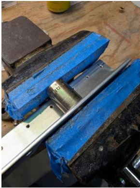
Using vice to press in symmco bushings
