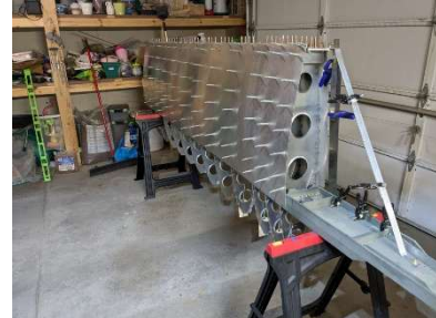
Aft skins pilot drilled
