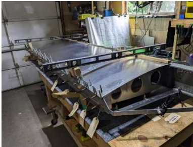
Starting to pilot drill LH upper aft skin
