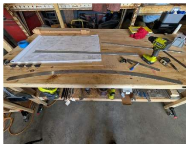
Centerline and offset marked on bow strap
