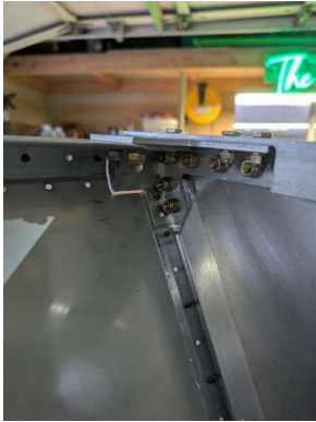
Hardware installed in RH upper motor mount
