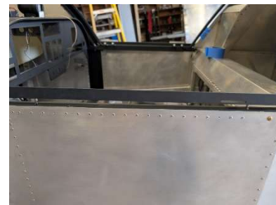
Alignment pins installed in canopy frame
