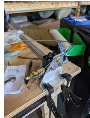
Testing out parking brake cable assembly
