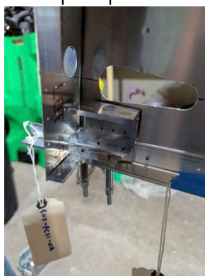
RH lower splice plate pilot drilled
