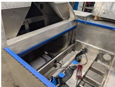
Interior components masked
