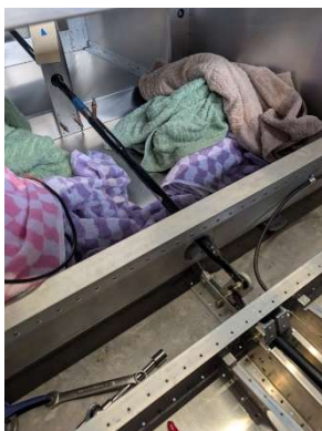
Forward pushrod support clecoed and pushrod halves pilot drilled
