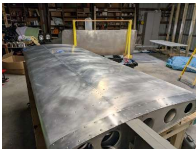
LH wing scotchbried and wing doubler riveted
