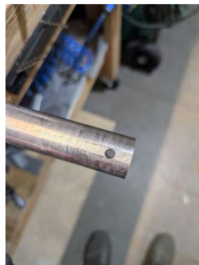
Hole drilled through main gear leg
