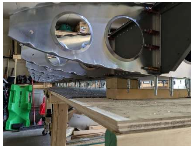
LH aft lower wing skin clecoed in place
