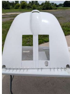
Exhaust tunnel outlets cut
