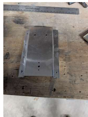
Mount plates bent and drilled
