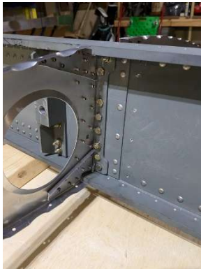
LH forward root rib installed
