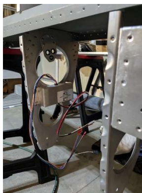
#4 rib installed with pitot heater controller
