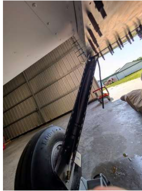
Gear leg fairing bolted to Adel clamps
