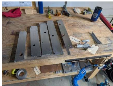
Vertical channels prepped for final assembly
