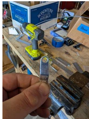
Enlarged hole in ball valve handle for cable nut
