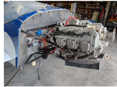
RH CHT and EGT sensors installed and wiring cleaned up
