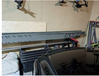
LH main spar partially riveted
