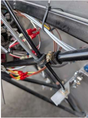
Throttle and mixture cables secured
