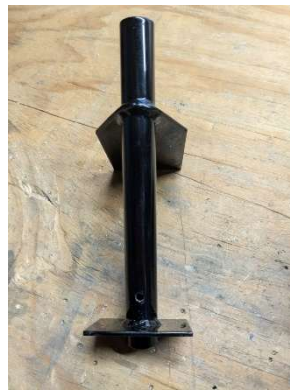
Pilot hole drilled in lower side of tail wheel mount
