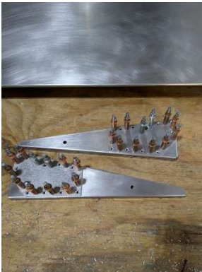
Drive ribs clecoed
