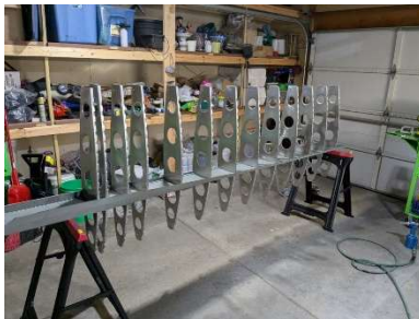
LH rib installation complete
