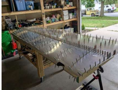
LH upper side updrilling in progress
