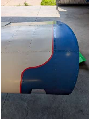
Tape applied to wing surfaces
