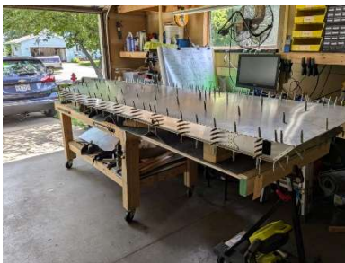
Flap and aileron hinge halves clecoed
