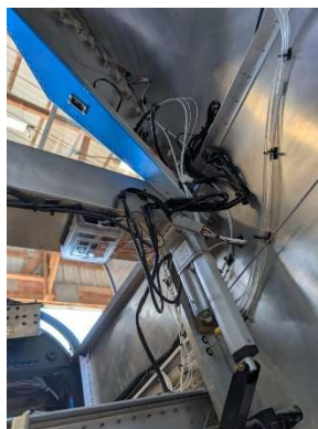
RH seat heat harness wired
