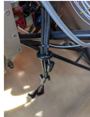
Spark plug grommet installed on harness
