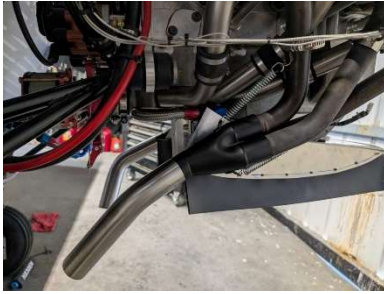
Exhaust pipes installed
