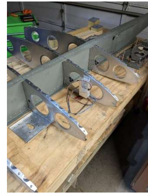
Pitot setup in forward part of wing
