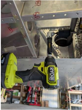
Pilot drilling forward wing attach angles
