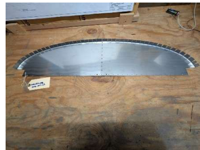
Assembly of -03 upper firewall former assembly
