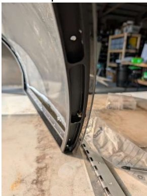
Through screw and nut installed in wallowed hole
