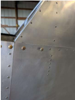
JB welded holes in side skin
