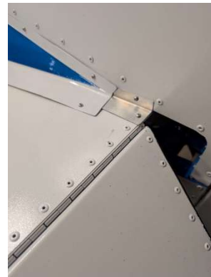
Fairing angle installed
