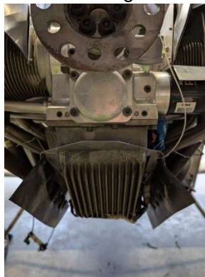
Oil cooler baffle temporarily supported
