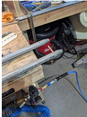
Drilling holes for pushrod ends
