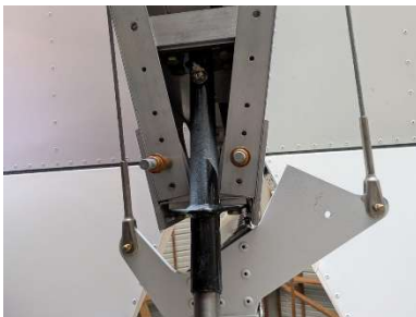
Tail spring epoxied into place and hardware installed
