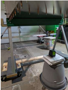
Laser level for setting axle height
