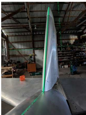
Elevator horn filed further
