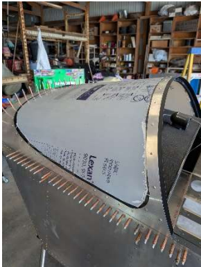
Screws installed in windshield and windshield bow
