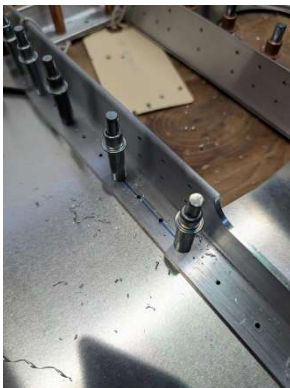
Extra holes drilled in wing angle per plans
