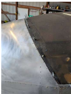
RH aft side canopy final fitment
