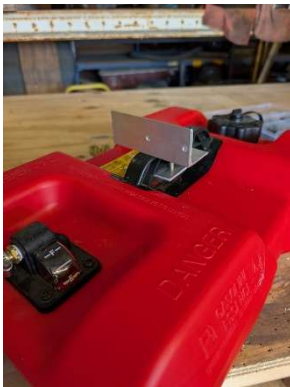
Component mount bolted onto tank handle
