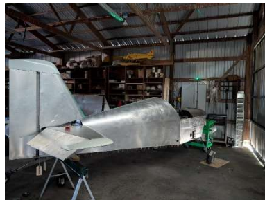
Rudder temporarily installed
