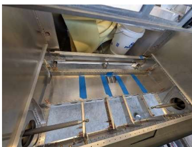
Rear spar carry-through temporarily installed
