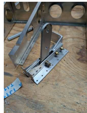
Brackets riveted to idler assembly
