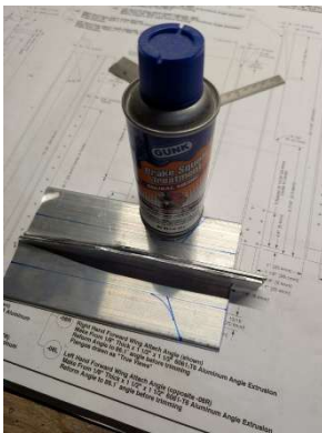
Using can to mark radii on -12 angles
