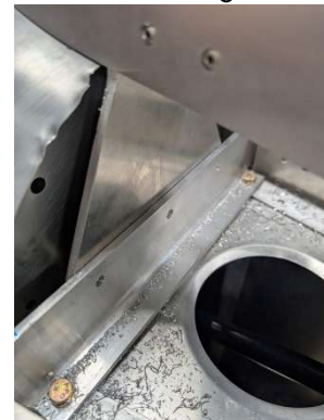
Forward mount holes updrilled
