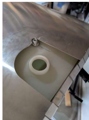
Trimmed glareshield so fuel vent fitting would fit better
