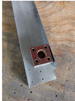
Cable fairlead blocks riveted
