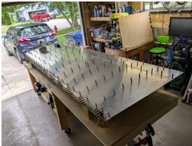
RH upper forward skins updrilled
