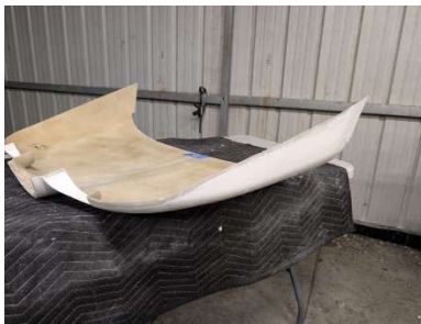
Upper cowl sanding in progress
