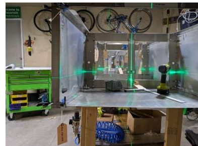
Forward pushrod support located via laser
