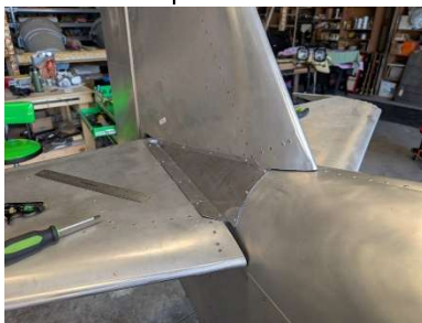
RH fairing panel installed
