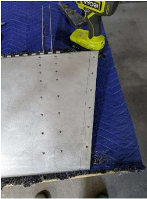
Top side of aileron with trim line
