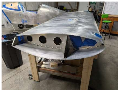
LH wing openings covered
