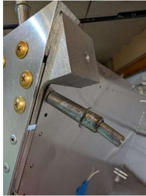
Interference between lower firewall and upper motor mounts.
