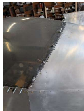
Aft side of canopy final fitment
