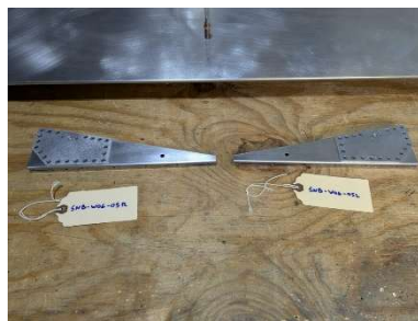
Front side of completed drive ribs
