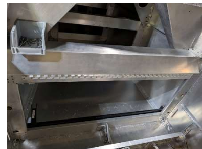
Hinge Half riveted
