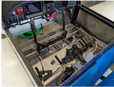
Forward floor removed
