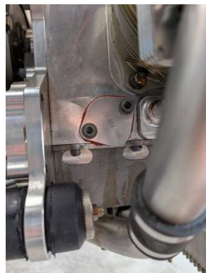
Block off plate installed
