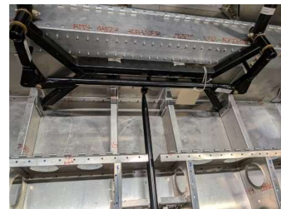
Idler bar temporarily installed on stick frame
