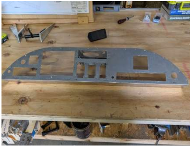
Panel cutouts complete
