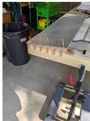
RH aileron tip rib updrilled
