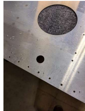
LH tie down bolt hole updrilled to 3/4"
