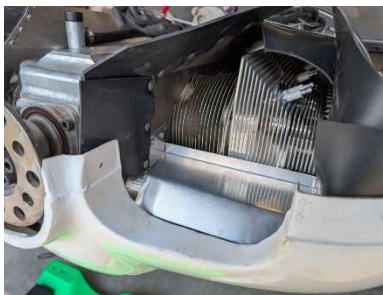
LH baffle plate installed
