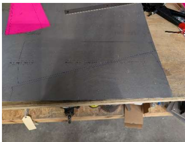
Transferring template to aluminum sheet
