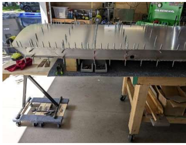
Aileron hinge half pilot drilled
