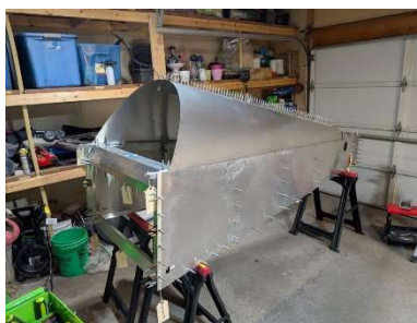
Turtledeck skin inserted in between side skins and upper longerons
