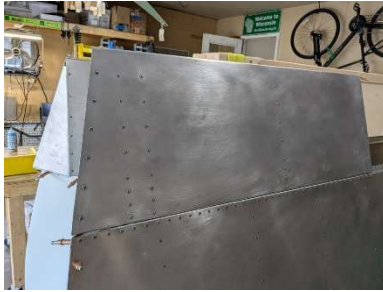
RH aileron installed on RH wing
