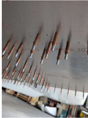
Master cylinder bracket clecoed to forward fuselage floor
