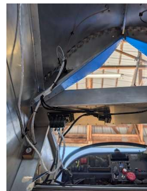
LH seat heat harness wired
