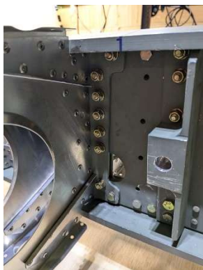
RH root ribs installed
