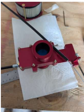
Throttle cable installed
