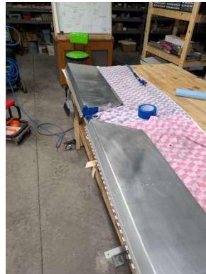
Elevator prepped for paint
