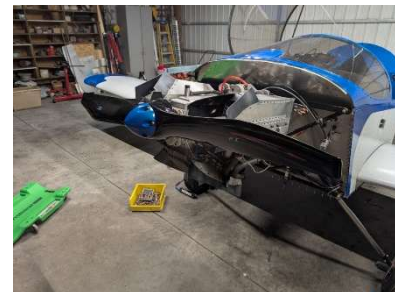
Prop and spinner installed
