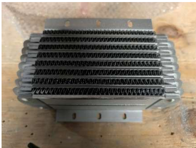
Bottom front tab removed from oil cooler
