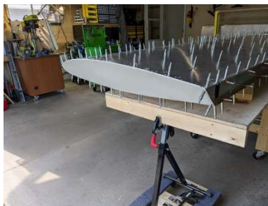
LH wingtip pilot drilled
