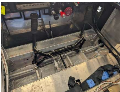
Stick grip harness wiring in progress
