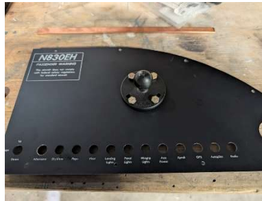
Ram mount base installed
