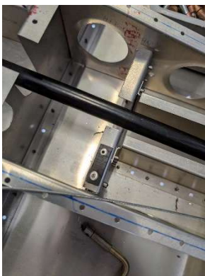
Cable slide plate riveted
