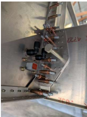
Pitot and AOA tube connectors mounted
