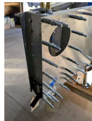
Pilot drilled RH side of aft fuselage channel
