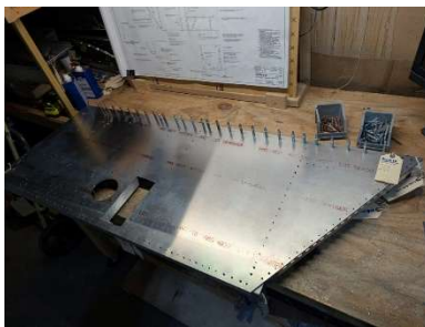
RH fuselage side panel updrilled
