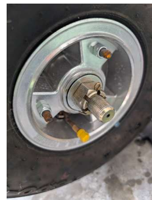
Cotter pins installed in axle nuts
