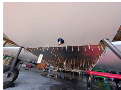
Lower cowl mount hinge partially drilled
