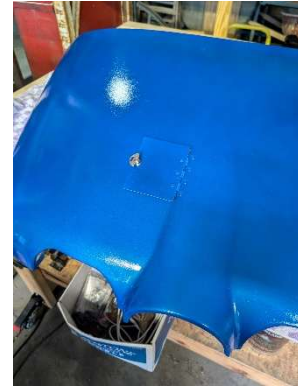
Oil door installation complete
