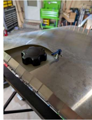
Fuel vent fitting installed
