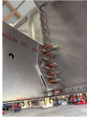
LH main wing attach angle drilled
