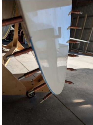
Filling gap between wing tip and wing skin
