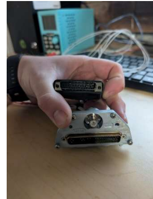
D-sub pins installed
