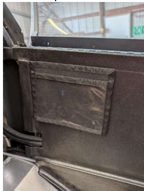
Document holder installed
