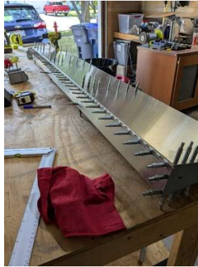
RH flap pilot drilling complete
