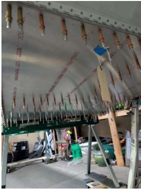
Fuselage floor clecoes
