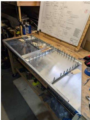
RH side panel clecoed with longerons and misc. angles
