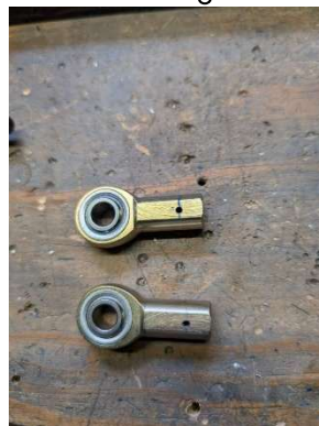
Drilling witness holes into female rod end bearings
