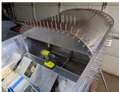
Instrument Panel updrilled
