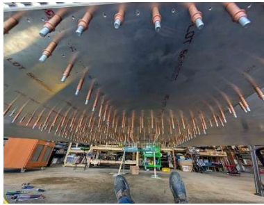
Fuselage floor clecoed on and forward spar web updrilled
