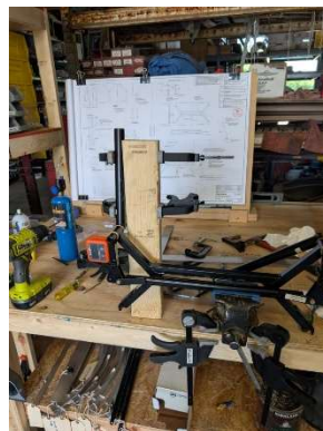
Using 2x4 to keep control stick vertical during shaft drilling
