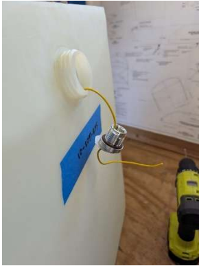
Used wire to fish fitting into place
