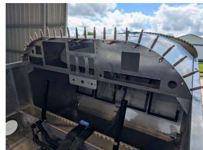
Temporary #6 screws installed in panel
