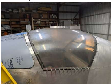
Canopy almost installed
