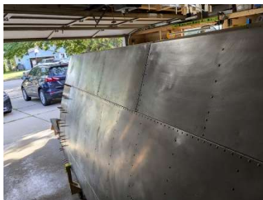
LH flap assembly installed
