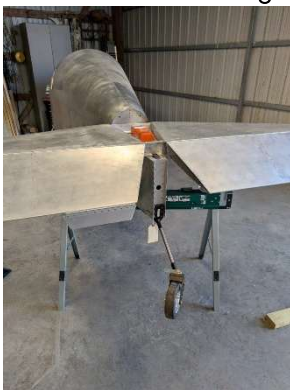
Inboard ribs drilled out and removed from elevator
