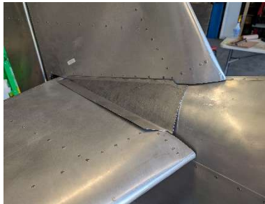
Rechecking fit after annealing
