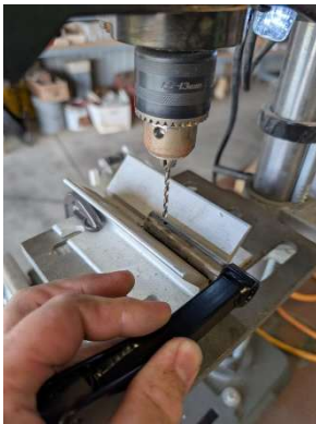
Drilling horn shaft for taper pin
