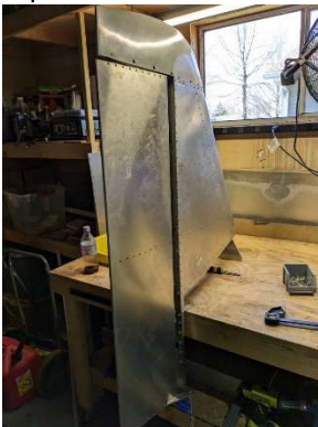
Completed vertical assembly
