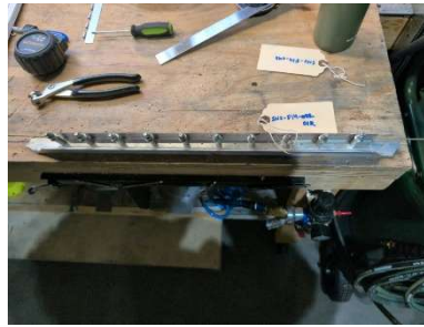
-01R forward angle assembly pilot drilled and complete
