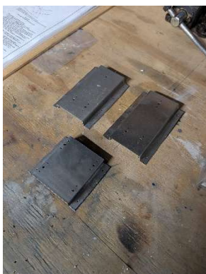
Mount plates complete with nut plates
