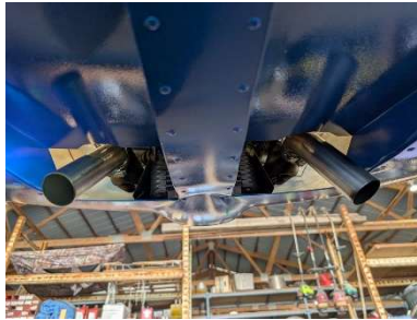
Exhaust pipes reinstalled
