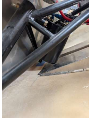
Interference between oil separator and exhaust tunnel
