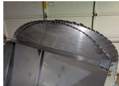
Firewall angle riveted
