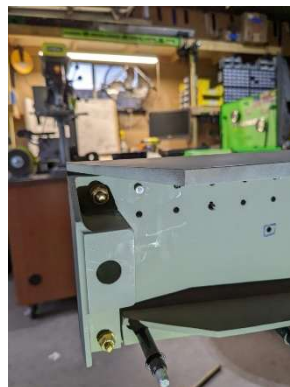
Wing attach block bolted
