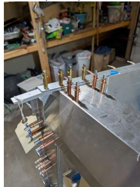
Updrilling upper splice plates and crossie box for AN3 hardware
