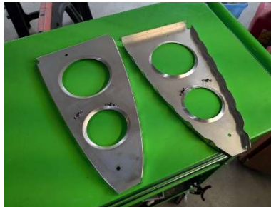
Outboard ribs with nutplates installed
