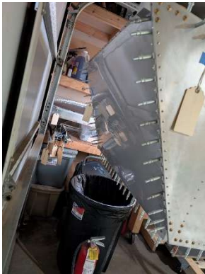
Lower firewall located and pilot drilled
