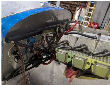
Starter motor installed and wire run along breather tube
