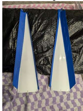
Tail fairing panels taped and prepped
