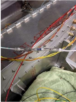
1.21k resistor in between GPS175 serial line and transponder
