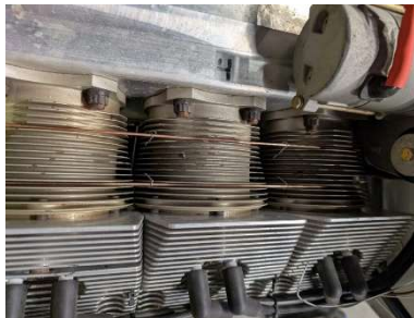
Baffles hung with welding rod
