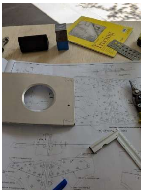
Layout of LH root rib
