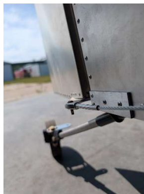
Clevis bolts temporarily installed
