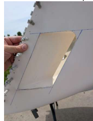
Test fit of cowl vent
