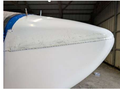
Marking trim reference line on RH side
