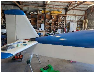
ELT antenna mounted to fuselage
