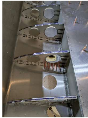
Access hole cut
