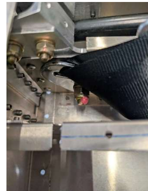
Torque seal applied to seatbelt hardware
