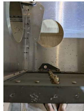
Wing tie down partially drilled
