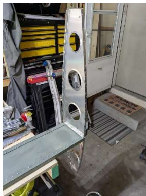
Rib installation starting from outboard side
