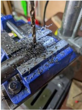
Drilling axle hole on drill press
