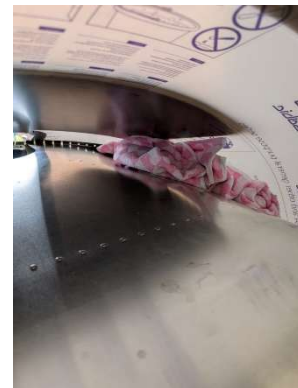
Towels stuffed between windshield and glareshield to "bow out" windshield to skirt
