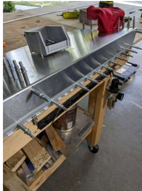
LH flap hinge half pilot drilling in progress
