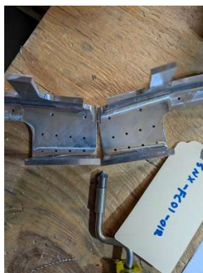
Holes drilled in vertical sides of splice plates
