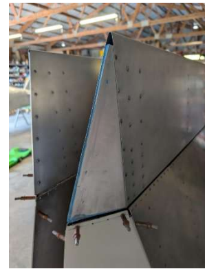
SuperFil used on aileron tip rib
