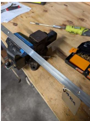
Countersunk inside holes for flush bolts
