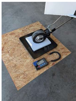
Tail wheel scale setup
