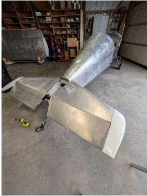
Horizontal tail assembly bolted into place
