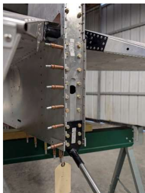
Lower rudder hinge half updrilled
