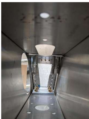
T12-05 angle holes drilled through upper longerons
