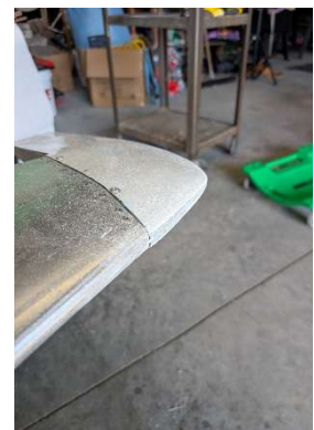
LH tail tip leading edge contoured
