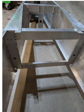
#3 cross ties and seatbelt mounts riveted
