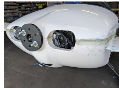
Fiberglass added to inlet ledges
