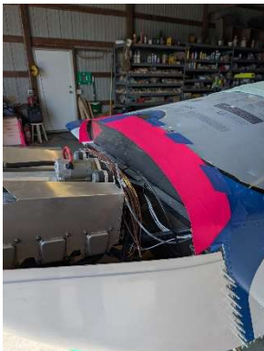
Tracing skirt geometry onto poster board
