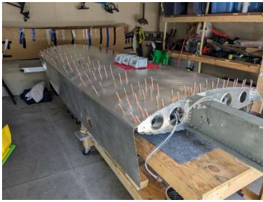
RH upper forward skin riveting in progress
