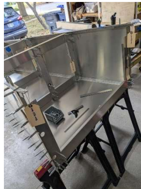
Both upper splice plates pilot drilled to upper longerons
