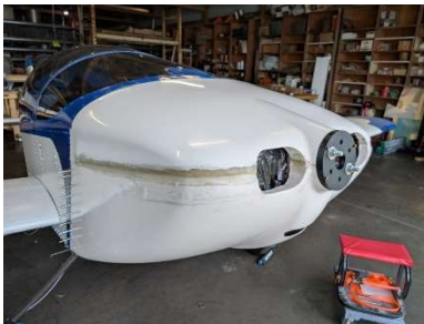
Fiberglass added to LH side of upper cowl
