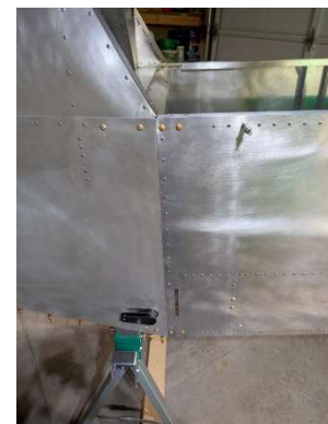
RH side panel riveted and hardware installed
