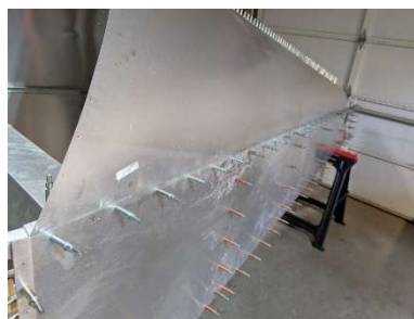
LH turtledeck skin partially pilot drilled
