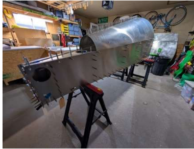
RH side panel updrilled
