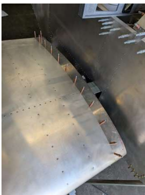
Marking doubler location onto RH wing
