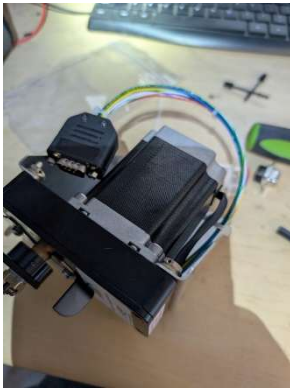
Connector added to roll servo
