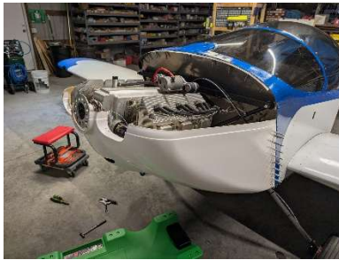
Prop and spinner removed and lower cowl installed
