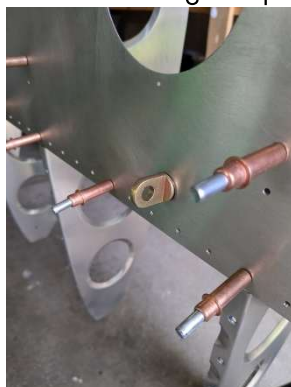
RH tie down bolt installed
