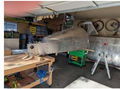
Placement of aft fuselage to enable underneath access
