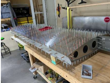
LH upper wing skin partially drilled
