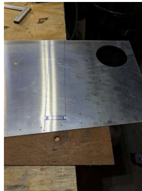
-01R cable hole laid out
