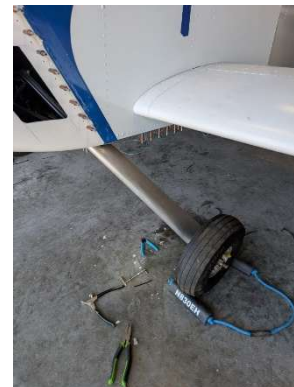
LH gear leg fairing installed
