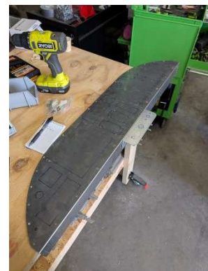
Panel blank marked for cutting
