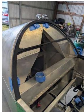
Canopy frame located with help from spacer blocks
