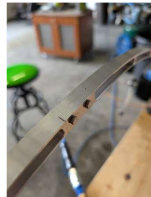
Solid -6 rivets installed
