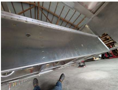
Rigging holes upsized
