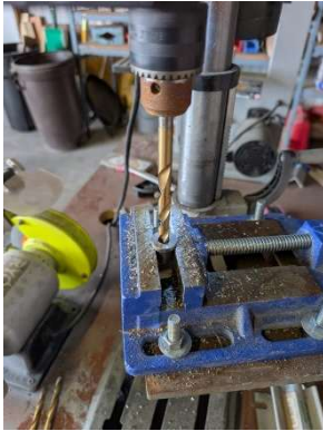
Enlarging holes in prop bushings
