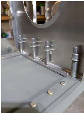
Main Spar – center spacer – web spacer – aft rib
