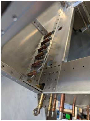
RH attach angle updrilled
