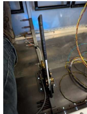
Brake handle installed
