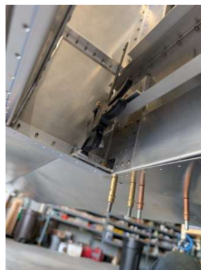
Setting incidence angle using clamps
