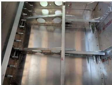
Seat ribs and channels pilot drilled to floor
