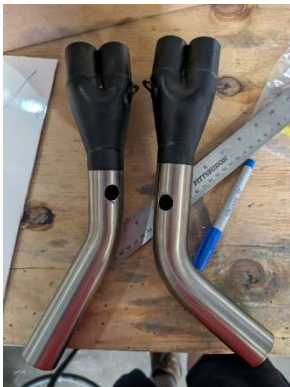
Holes drilled in exhaust pipes
