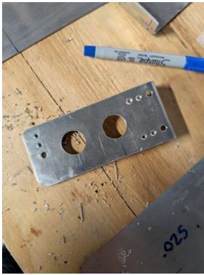
Drilling holes for nutplates
