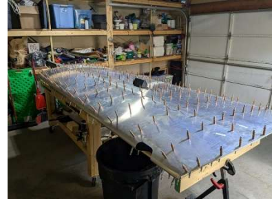
LH wing upper wing skins updrilled
