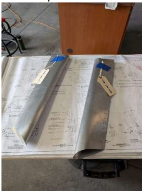
Marking bend for annealing process
