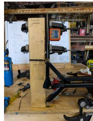
Using 2x4 to keep control stick vertical during shaft drilling
