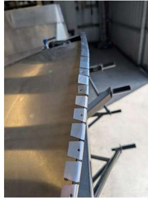
Upper firewall holes deburred
