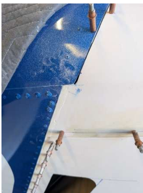
Sanding aft edges of upper cowl on aircraft
