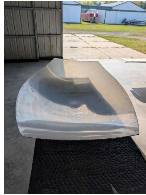
Canopy removed and edges sanded
