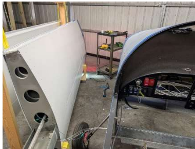
LH wing lighting test
