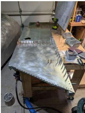
RH forward side panel rivets installed
