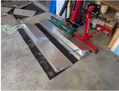
Ailerons and flaps removed from wings
