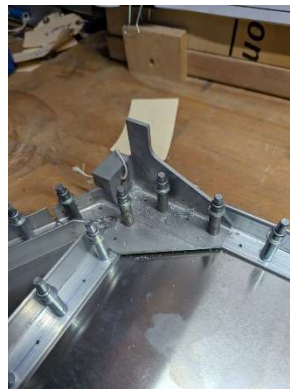
LH lower motor mount located and pilot drilled
