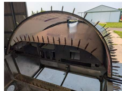
Windshield bow inserted and pilot drilled to windshield
