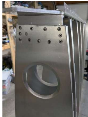
LH aft root rib riveted to rear spar
