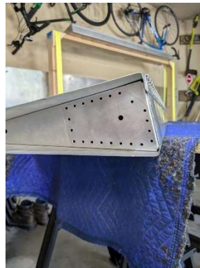
Legacy flap drive plate removed
