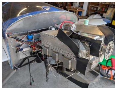
RH baffle installed
