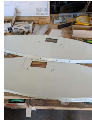
Access holes cut in wingtips
