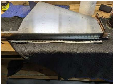
Hinge half rivets drilled out
