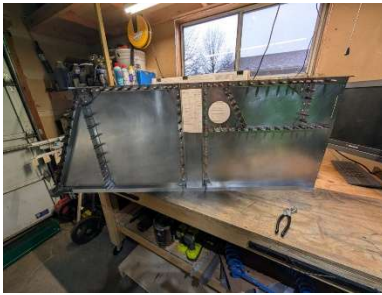
LH forward side panel clecoed together
