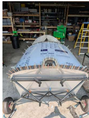
Upper firewall skirt holes updrilled
