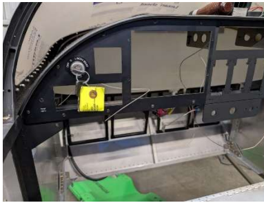
LH panel installed
