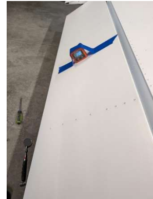
Calibrating flap position sensor
