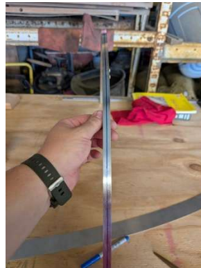
Centerline marked on windshield bow
