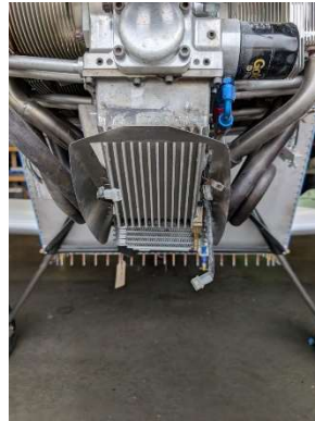
Oil cooler remounted higher
