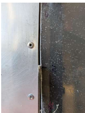
Checking clearance between canopy and fuselage
