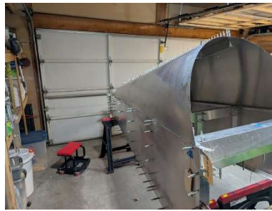
RH side turtledeck skin located and partially pilot drilled/clecoed
