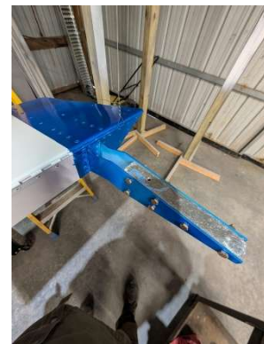
Drilling out LH aileron counterweight
