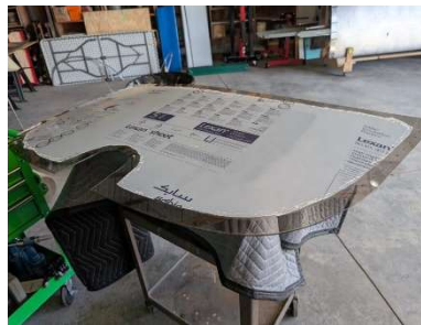
Windshield holes updrilled
