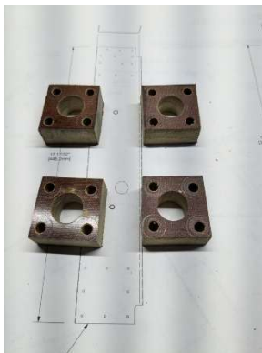
Center hole updrilled. -.09 blocks complete.
