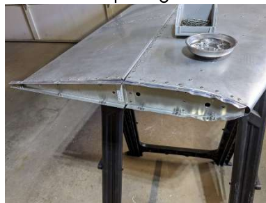
RH tip final riveting
