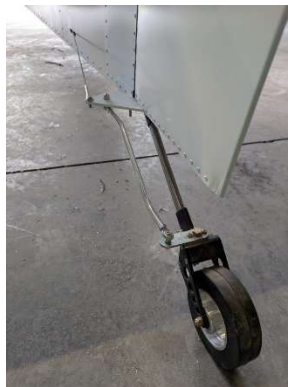
Anson Engineering steering rod installed
