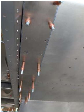
LH wing root doubler clecoed into place
