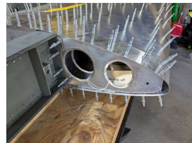
LH forward Root rib pilot drilled
