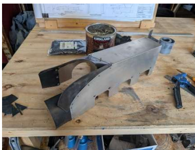
Cutting and riveting rubber baffle material
