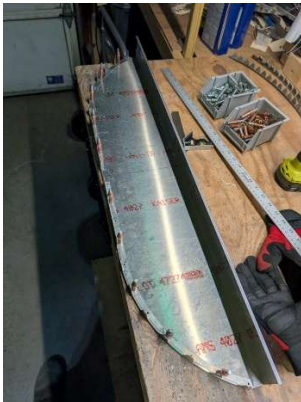
-02 instrument panel assembly clecoed
