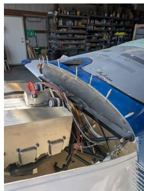
Upper cowl shelf installed with spacers
