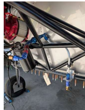
New fuel line installed
