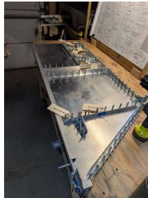
RH fuselage side panel pilot drilled
