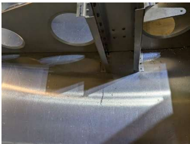
Aileron bellcrank support angles drilled to lower skin
