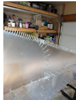
Former #3 clecoed into place
