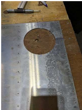
-01R rudder access hole cut
