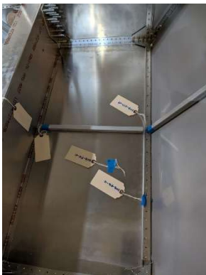
Floor stiffener pilot drilled
