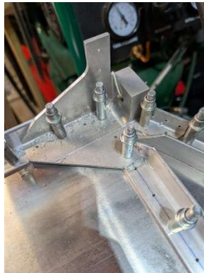
Lower motor mount located and pilot drilled
