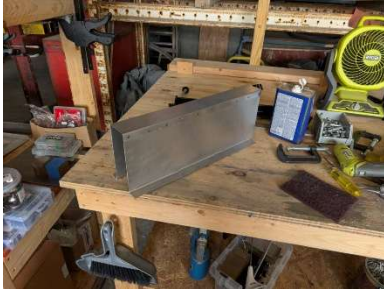
Elevator pushrod cover fabricated
