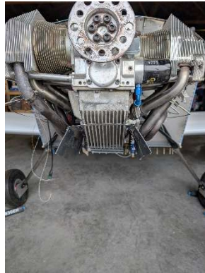
Oil cooler baffling installed
