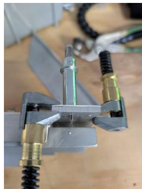
F03-07 spacer being located on rear spar carry through
