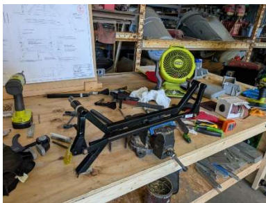
Link rod installed onto stick horns
