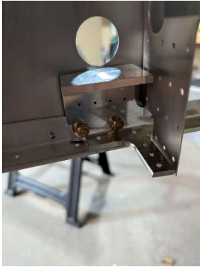
AN525 hardware installed in splice plates
