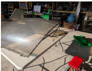
Canopy being attached to frame
