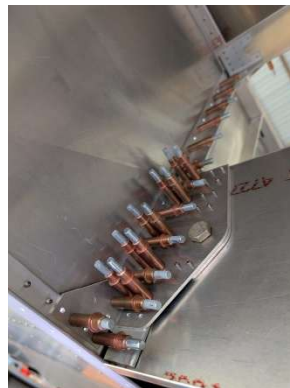
RH main wing attach angle drilled
