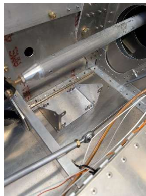
Test fit of roll servo bracket
