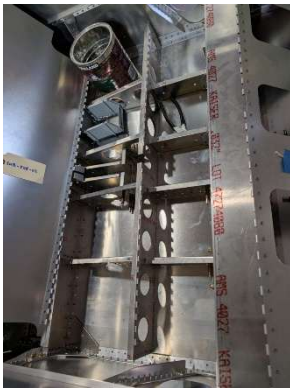
Hinge halves riveted to seat pan channel
