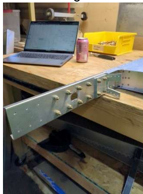
Vertical stabilizer spar
