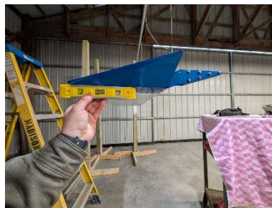
Checking levelness with counterweight attached
