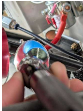
Setting needle height via sharpie mark
