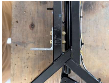
Pitch servo bracket bolted to control frame
