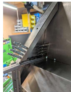
RH former clip pilot drilled
