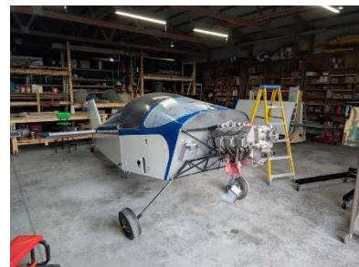
Engine temporarily mounted
