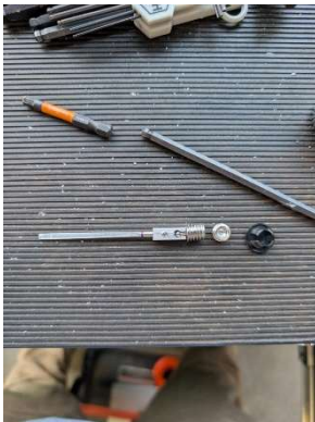
#3 AeroInjector needle installed in carrier
