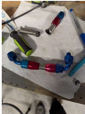
Short fuel line between fuel filter and AeroInjector
