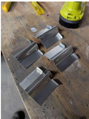
Baffles cut, bent, and drilled
