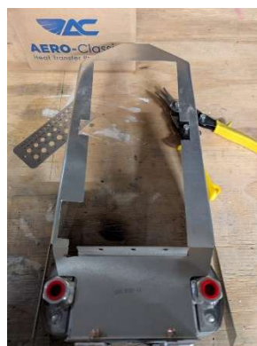
Oil cooler baffling notched
