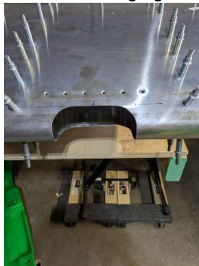
Holes drilled for upper lens retainer
