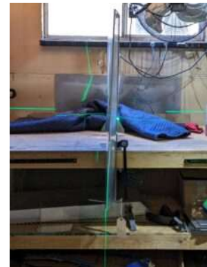
Verifying rudder alignment with laser
