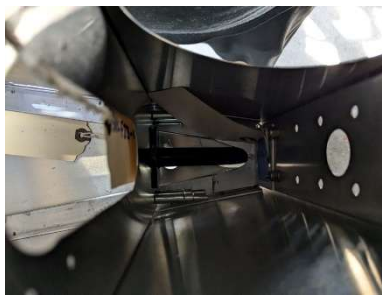
Note gap between tail wheel mount and rear bulkhead on LH side of picture
