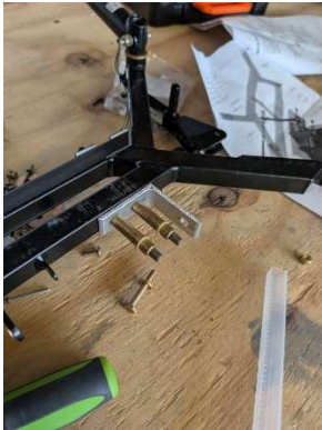
Test fitting autopilot bracket
