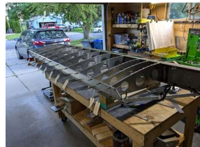
Rear spar locked square
