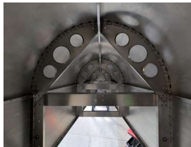
#2 formers riveted to tail cone box and skin splice channel
