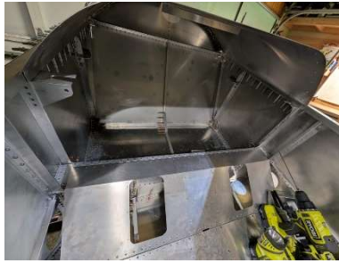
Glare shield pilot drilled
