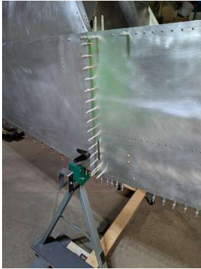
RH splice plates pilot drilled
