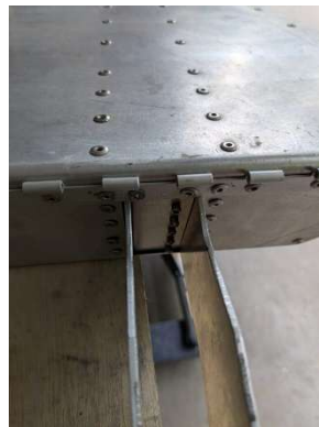
-06L hinge half rivets finished
