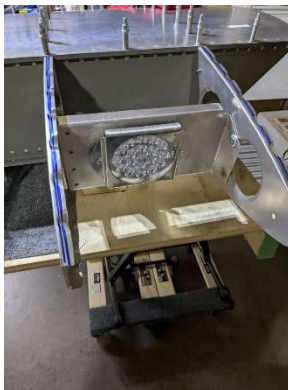
LH light assembly mounted into wing aimed full down
