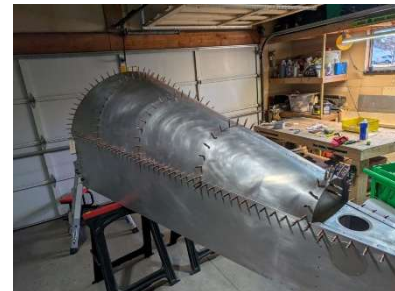
Formers #4 through #2 clecoed into place
