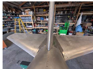
Fairing panels final fit
