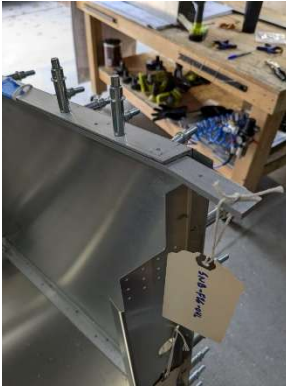
LH upper splice plate located
