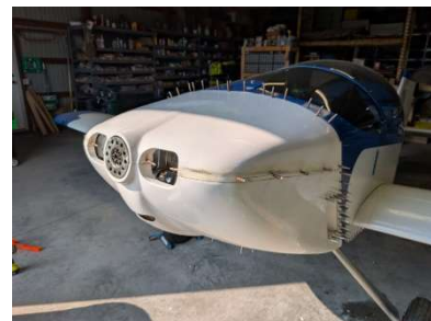
Upper and lower cowl fit onto fuselage
