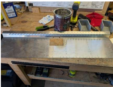
Rear seat pan riveted and deburred
