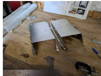
Exhaust tunnels bent
