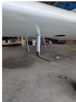
Pitot probe installed
