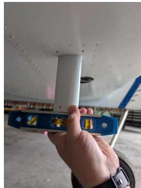
Pitot mount alignment verified
