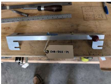
Canopy latch assembly complete
