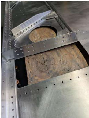
LH rear wing attach angle countersunk
