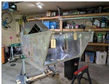
Upper forward cross tie clecoed
