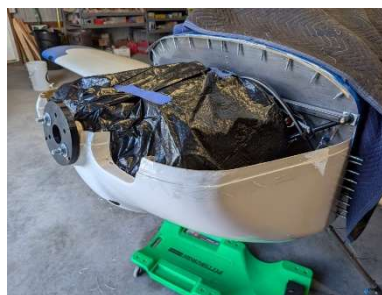
Engine covered and overlap of lower cowl taped
