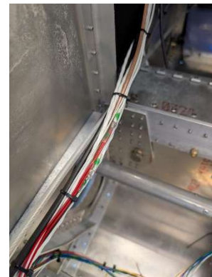
Autopilot grounds and powers spliced
