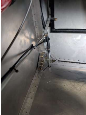
Forward floor bolts installed
