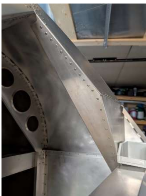
LH former strap riveted
