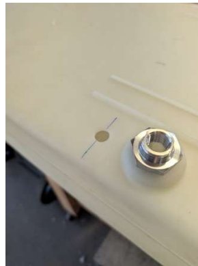
Fuel sender hole drilled
