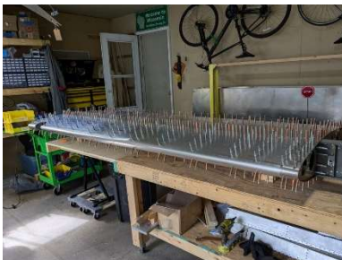
LH underwing updrilling in progress
