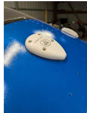
Both GPS antennas mounted
