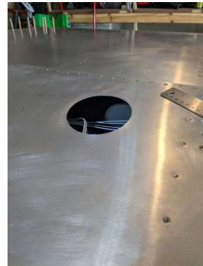
Pitot inspection plate holes drilled
