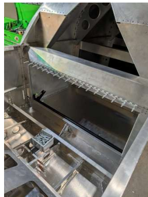
Upper seat back hinge half pilot drilled
