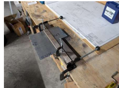
Bending battery box
