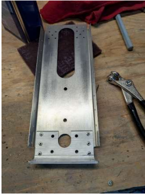
Riveted lower aft angle to aft bulkhead
