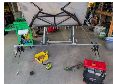
Aluminum angle used to set axle toe in
