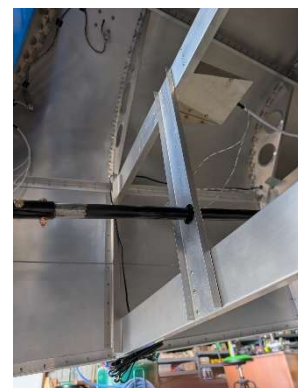
Forward push rod assembly riveted
