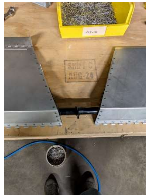
Elevator rework complete
