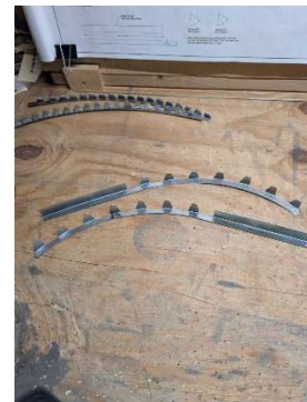
Instrument Panel angles bent
