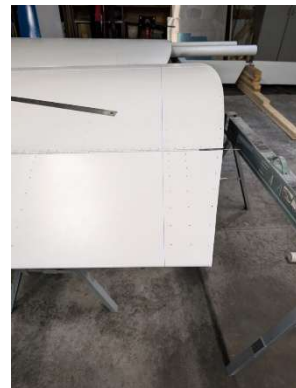
Projecting lines onto ailerons
