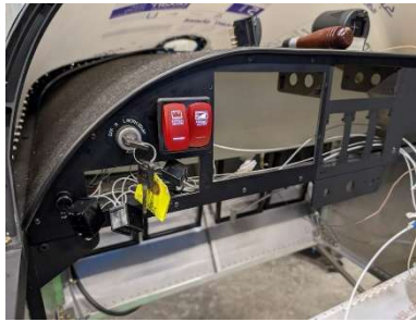
Panel dimmer and two switch gang wired and installed into panel
