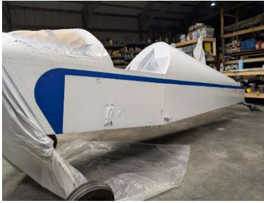
Fuselage taped, prepped, and partially masked
