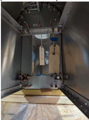
Aft fuselage station #5 updrilled
