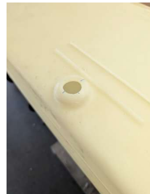
Main fuel drain hole cut
