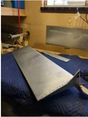
Rudder not laying flat on table
