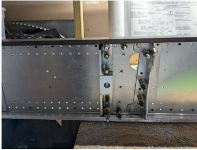
RH root wing attach assembly and root rib attach angle
