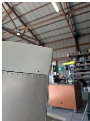
Aft edge of vertical tail tip slightly adjusted to align with rudder
