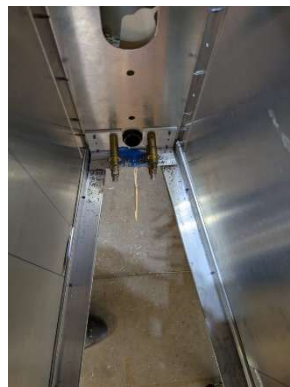
Replaced F23-02 and -03 aft bulkhead and lower angle and updrilled tail wheel mount holes to 3/16"
