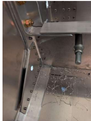
-02 assembly located and pilot drilled to RH forward fuselage
