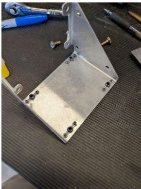
Nutplates installed in servo bracket
