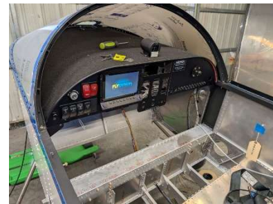
HDX screen temporarily installed and tested
