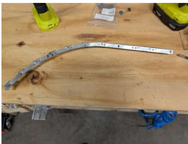
Nutplates installed in left panel flange
