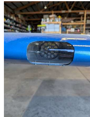
RH landing light lens installed
