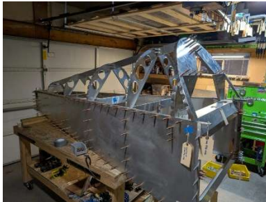
Turtledeck skin removed to updrilled skin splice channel
