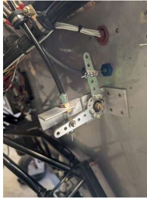
Throttle cable reinstalled and cable nuts tightened
