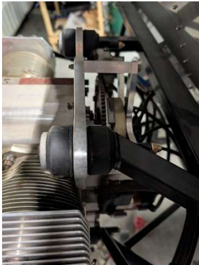
Engine mount hardware replaced with proper size
