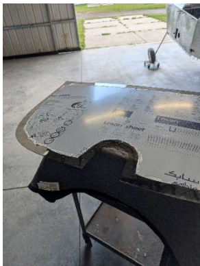
Protective film removed from edge of windshield
