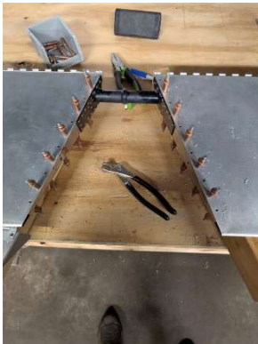
Inboard elevator ribs drilled
