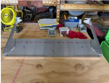
Forward tunnel zee removed
