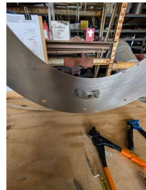
Southco receptacle installed
