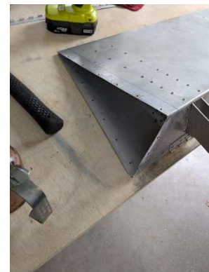
LH existing aileron tip rib removed
