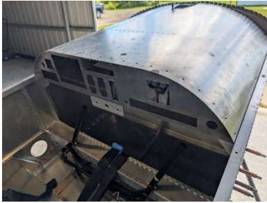
Panel blank and angles riveted
