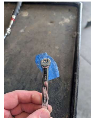
Nut retention technique
