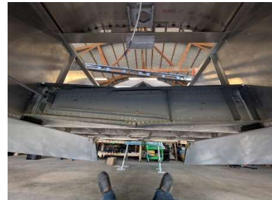
Spars pinned via rigging holes and centered with fuselage
