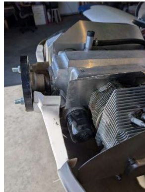
Cylinder baffles trimmed
