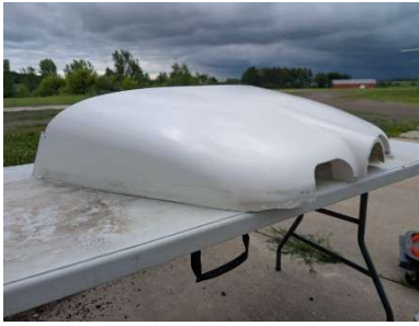
Rough sanding cowl curvature and transition line
