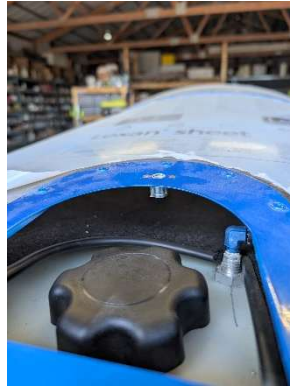
SkyBolt receptacle installed in windshield skirt
