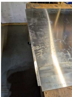
Forward fuselage floor aft edge bent 5 degrees
