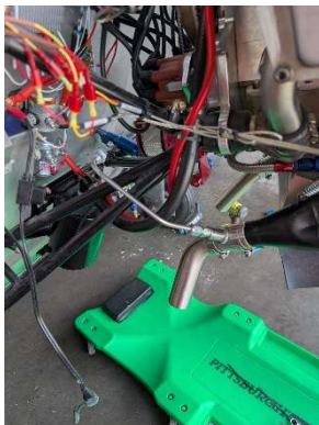
Fluid line routing through firewall
