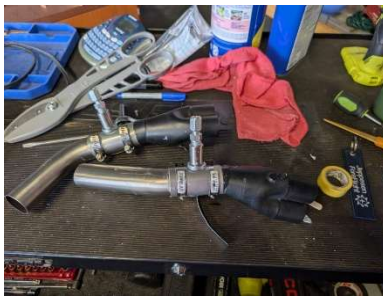
Sprayers attached to exhaust with worm clamps and exhaust sealant
