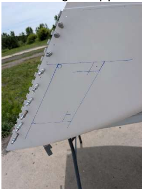
Cowl vent cut pattern laid out
