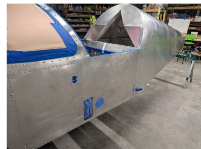
Fuselage openings taped
