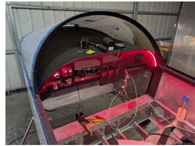
Panel light strip installed and tested
