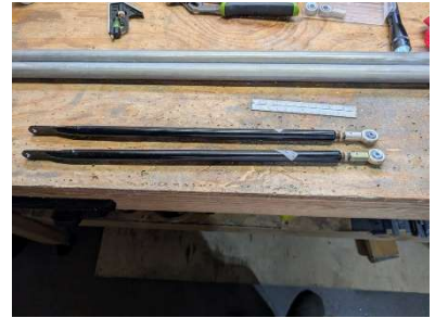
-02 aileron pushrods complete
