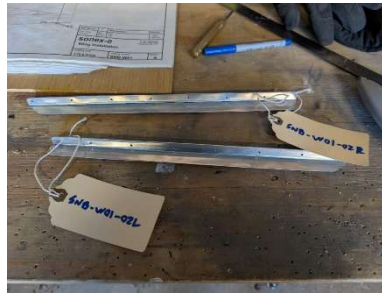
Flap fairings cut, bent, and drilled
