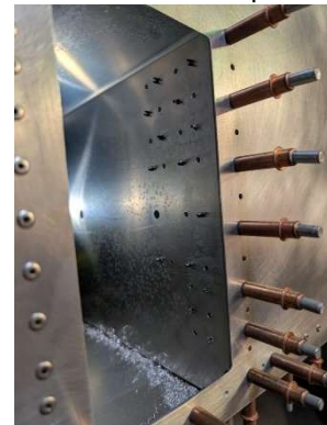
LH aft tunnel web updrilled
