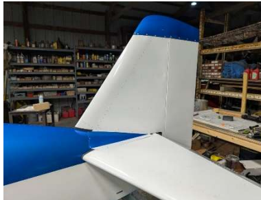
LH tail fairing panel installed
