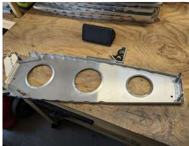
Ribs #1-4 trimmed and gussets installed
