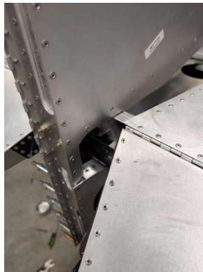
Elevator horn interference
