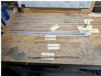
Seat pan hinges cut and pilot drilled
