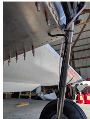
Fuel vent temporarily attached to LH gear leg
