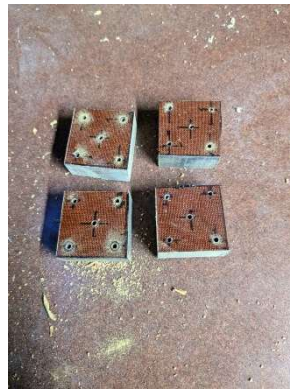
All holes pilot drilled
