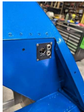
Pilot side headset jacks installed
