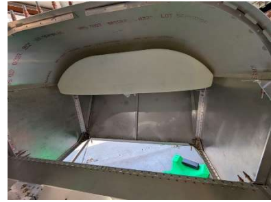
Tank mocked up into place
