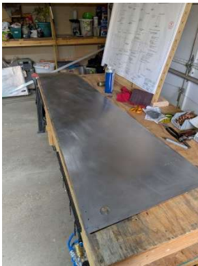
LH aft side skin deburred, scotchbritten, and cleaned
