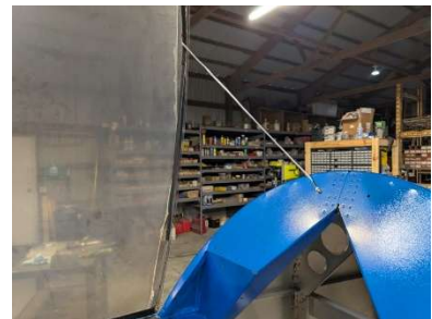
Canopy strap installed
