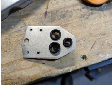
Pitot tubing/wiring support plate
