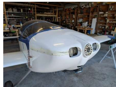
Checking cowl fitment with permanent fasteners
