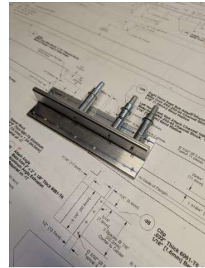
Transferring holes between -18 pivot angles to ensure alignment
