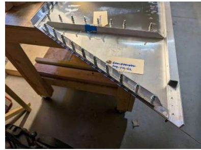
F14-01L assembly located and pilot drilled
