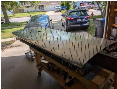
LH wing doubler (bottom) attached
