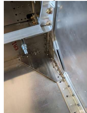
RH gusset and spacer located and pilot drilled
