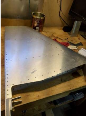
Previously completed vertical stabilizer
