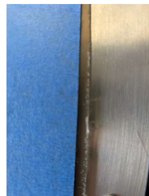
Marking rear trim line with tape
