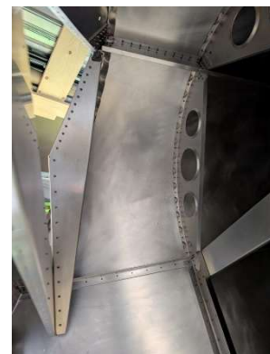
RH former strap riveted
