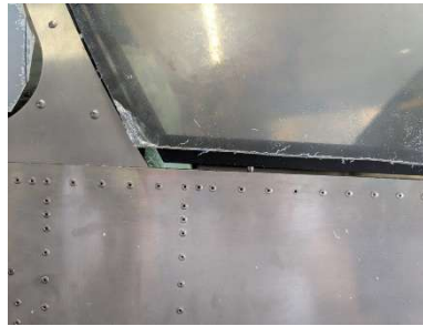
Canopy frame pulling up in front
