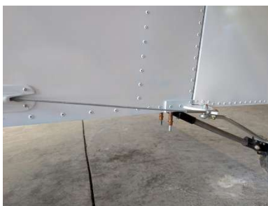
Rudder cables attached to rudder and fairings installed
