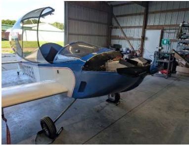
Lower cowl reinstalled
