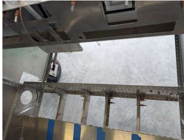
Forward tunnel zee removed
