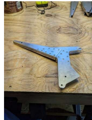
Rudder drive horn riveted
