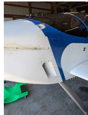
LH hinge half and cowl vent riveted
