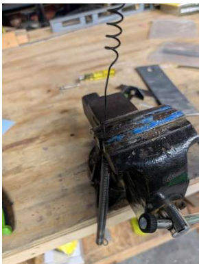
Bending spring steel with heat
