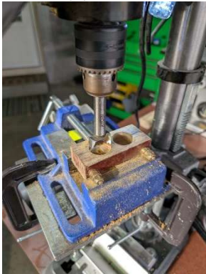
Drilling through holes
