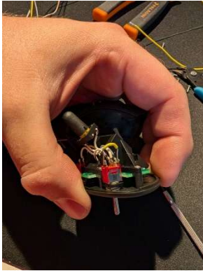
Resoldering stick grip switches to isolate PTT circuit
