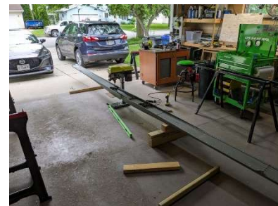
Wing attach block drilling process
