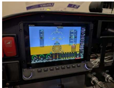
Mapping sensors and gauge layout on PFD
