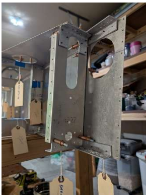
Updrilling aft bulkhead
