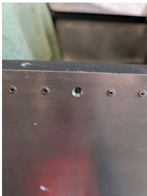
Latch pin holes countersunk
