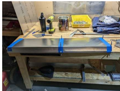
Clecoing rudder assembly together
