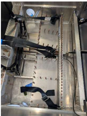
Aft seat pan clecoed into place
