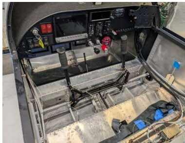
Ailerons rigged to control stick frame. Control installation complete!
