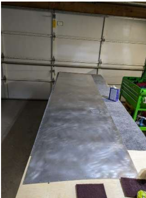
LH lower aft wing skin deburred and cleaned
