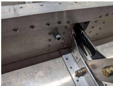
Conduit retainer installed below seat pan
