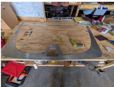
Windshield skirt updrilled and deburred
