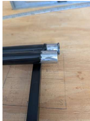
Removed powder coating from rudder pedals
