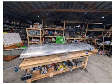
LH wing prepped for paint
