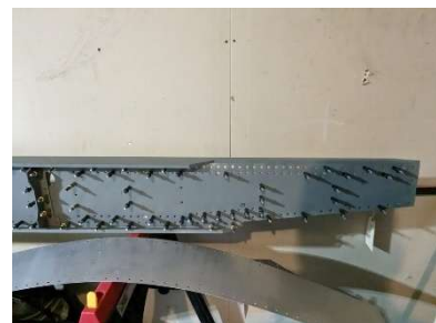
Flush rivets started
