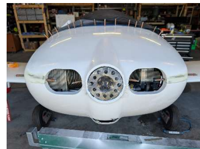
Adding micro to last couple spots
