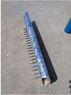
Marking bend for annealing process
