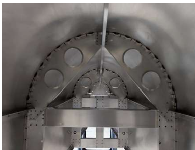
#3 formers riveted to tail cone box and skin splice channel
