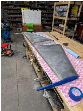
Horizontal stabilizer prepped for paint
