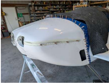
Using micro to fill low spots on new work
