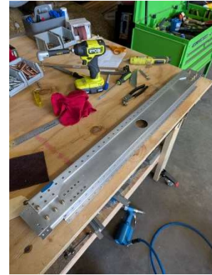
Shear web riveted onto rear spar carry through
