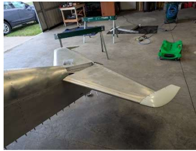
Horizontal tail assembly bolted into place
