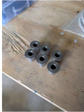
Prop bushings drilled for AN6 hardware
