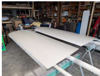
White wing paint complete
