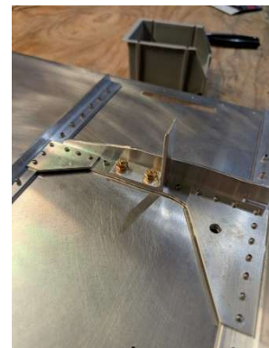
Seatbelt angle bolts installed
