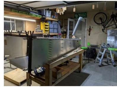
Testing tail fitment on aft fuselage section
