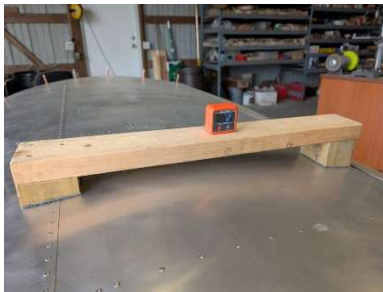
RH wing incidence angle being checked
