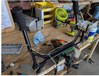
Wiring secured and terminated into Molex connector
