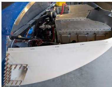
Nutplates installed in lower cowl
