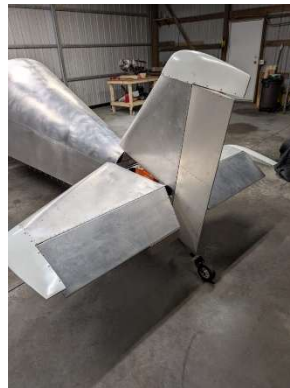
Tail components reinstalled onto fuselage
