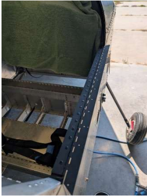
Hinge rivets installed and painted
