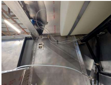
Routing wires loosely on LH side of forward fuselage
