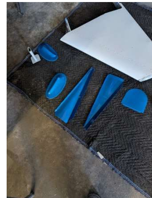
Fairing panels painted blue
