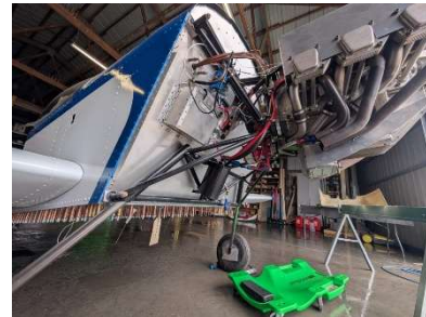
Cowl hinges mounted on firewall
