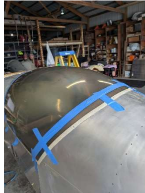
Rear trim line marked with tape
