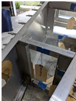
F22-06 angle fit and pilot drilled
