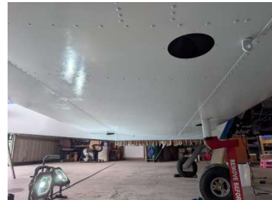
RH under wing color sanded and buffed
