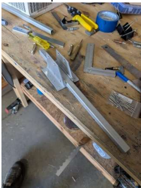
Master cylinder mount riveted to forward fuselage floor tube
