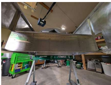
Aft spar tunnel web riveted
