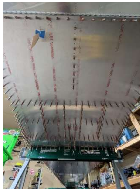
Forward fuselage floor deburred and clecoed
