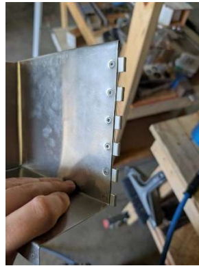
Flush rivets used on piano hinges
