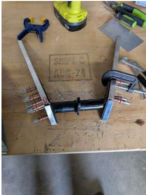
Inboard elevator ribs located and clecoed
