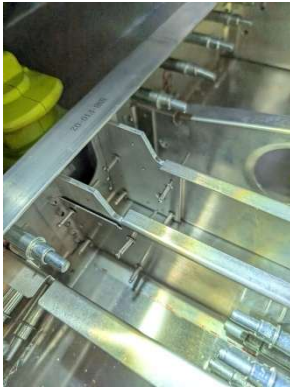
Used rivet stems to locate inner seat belt channels
