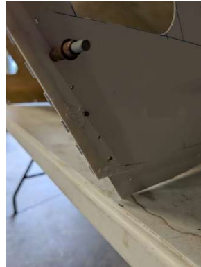
Adding micro to low spots on lower cowl
