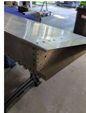
Location of new inboard rib on flap
