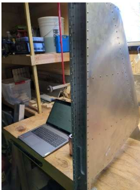
Previously built vertical stabilizer
