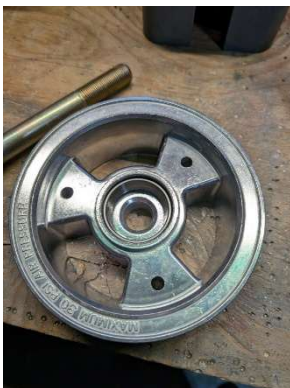
Bearing race pressed to proper depth
