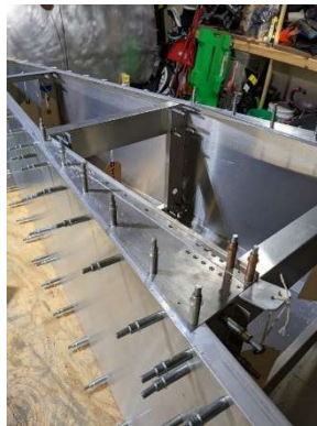
RH seat belt support installed
