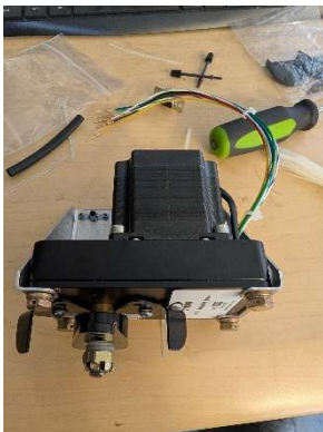
Pitch servo over-center bracket attached and d-sub pins crimped
