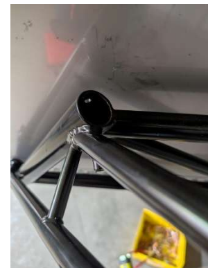
Gear leg hole drilled through
