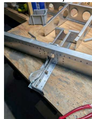
Center seat belt channel components riveted
