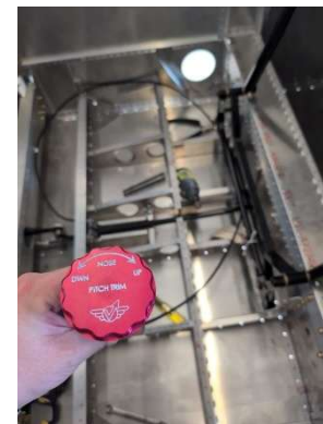
Forward spring installed and attached to trim cable
