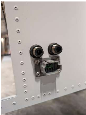
RH wing root connections installed
