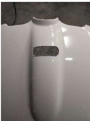
Oil cooler intake cut
