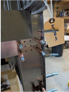
LH of crosstie box updrilled
