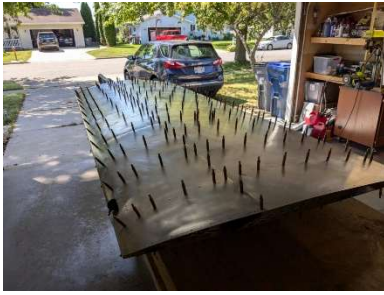
LH forward wing skin clecoed into place with root doubler
