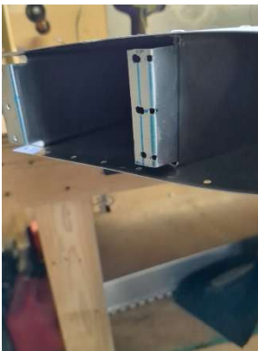
Hole issues in tip rib
