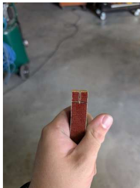
Flange tool out of scrap phenolic
