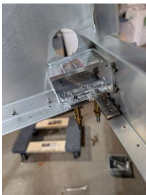
LH flap angle pilot drilled and clecoed
