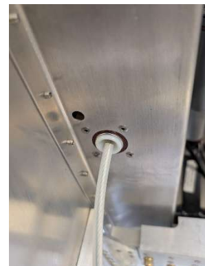
Forward fairleads installed
