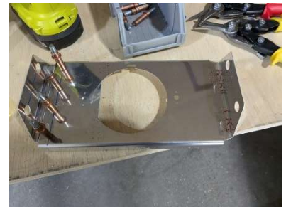
Mounting plate trimmed and clecoed together
