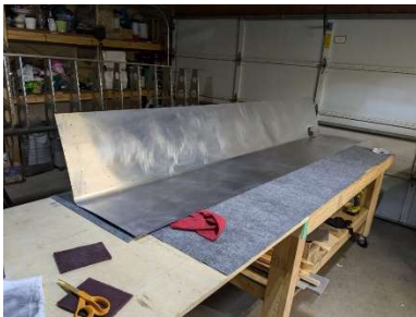
LH forward wing skin deburred and cleaned
