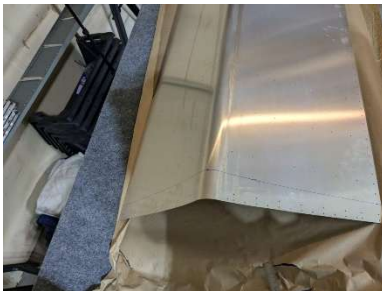
Trim line marked
