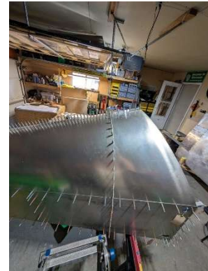
Former #2 clecoed into place
