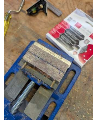
Pilot drilling through holes
