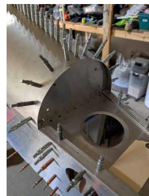
Former #5 pilot drilled and located
