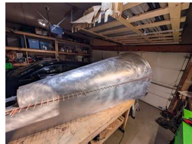
Formers #5 through #1 riveted to turtledeck skin assembly
