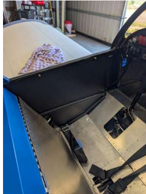
LH side panel installed
