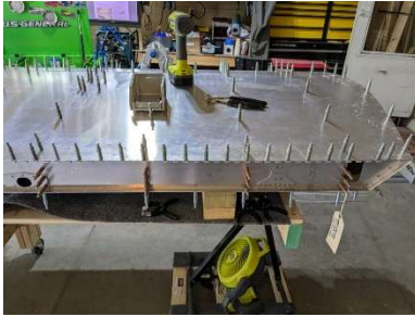
Aileron hinge half clecoed
