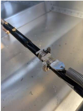
Clamp added to balance spring tab
