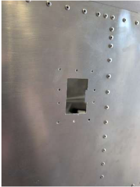
Vent cutout complete and cleaned up
