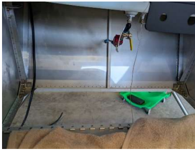
Removed forward floor and rudder pedals
