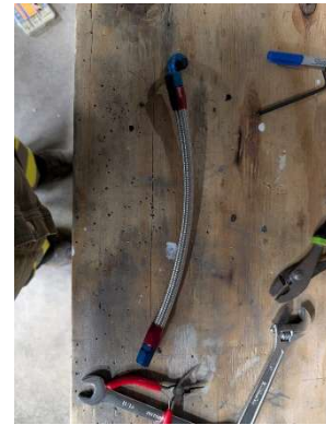
Oil cooler hose assembled
