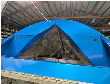
Headset panel holes drilled
