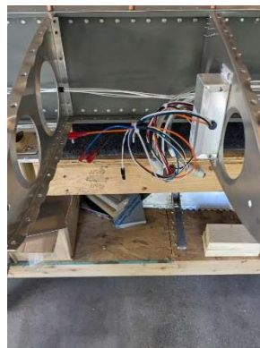
Pitot controller wiring and tubing runs
