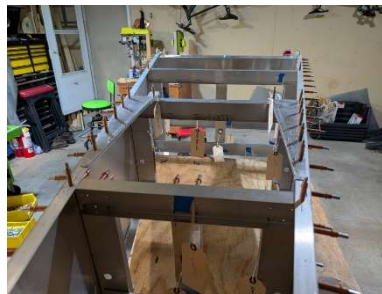
Aft mounts updrilled
