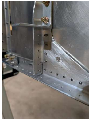
Fuselage parts deburred
