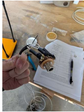
Copilot Mic jack soldered
