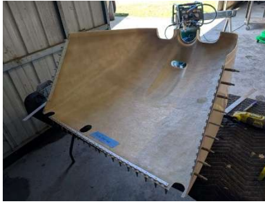
Mount hinge halves pilot drilled and clecoed
