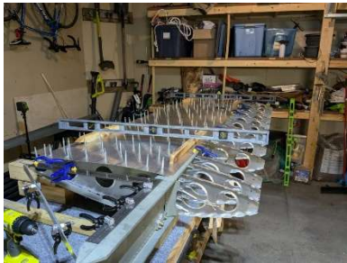
Lower aft skin pilot drilled
