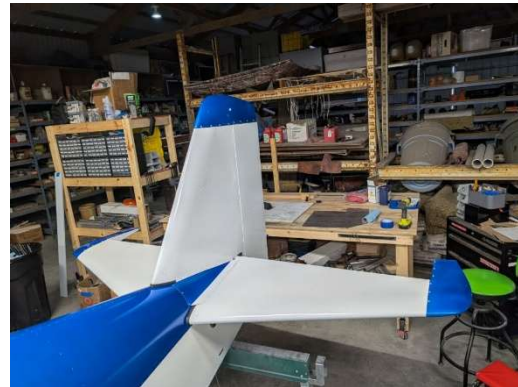
Tail tips installed
