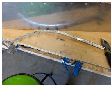
Began installation of nut plates on panel mount flange
