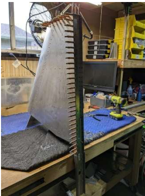
New hinge clecoed into place
