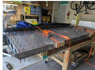
Ratcheting LH forward wing skin into place
