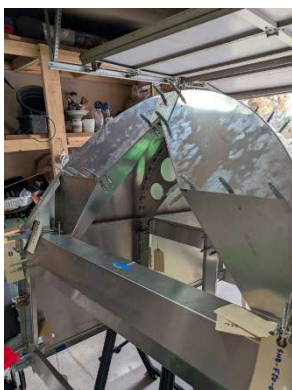
New #1 formers located and final drilled
