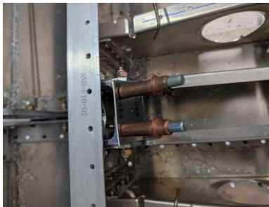
Seat support strap located and drilled
