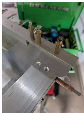
Upper forward cross tie updrilled and countersunk
