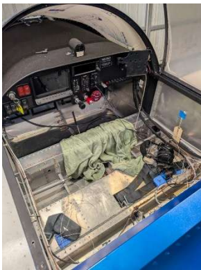
Wire routing cleanup in progress
