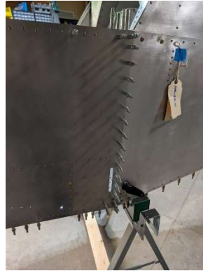
LH splice plates pilot drilled
