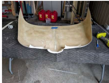
Upper cowl air intakes cut
