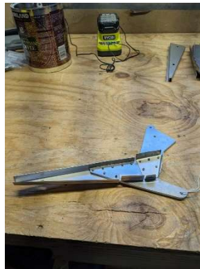
Rudder drive horn riveted
