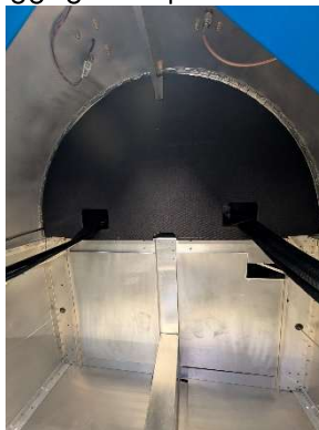
Baggage compartment covers installed
