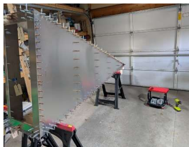
Aft fuselage floor updrilled
