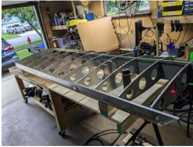
RH rib installation complete
