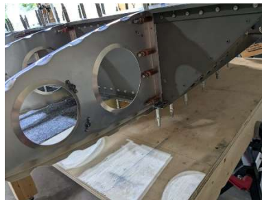
Ground lug nutplate installed
