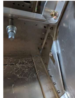
-02 assembly located and pilot drilled to LH forward fuselage
