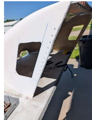
Aft cowl edge scarfed for extension
