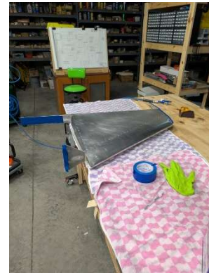
Vertical stabilizer prepped for paint
