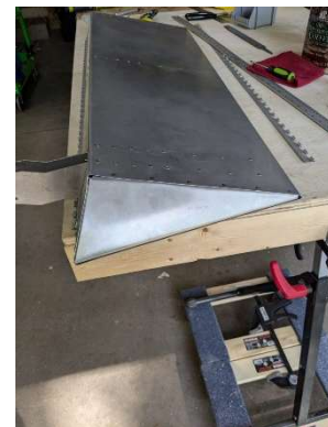
RH aileron tip rib riveted
