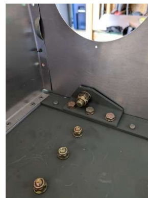
RH tie down bolt installed
