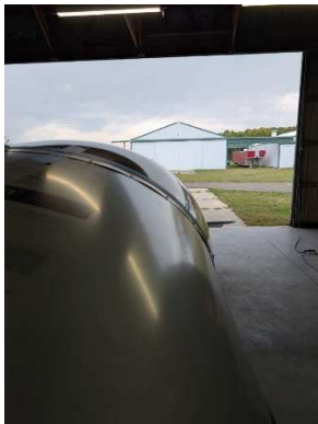
Canopy slightly bulging on sides
