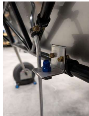
Drain cock assembly mounted
