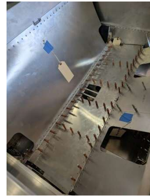
Lower seat back hinge half updrilled
