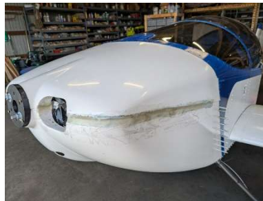
Fiberglass added to RH side of upper cowl
