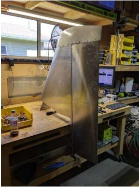
Completed vertical assembly
