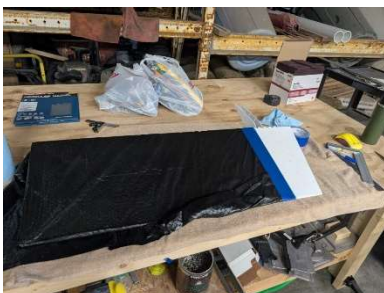
Ailerons prepped, taped, and masked
