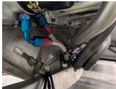
Oil cooler hose #2 installed
