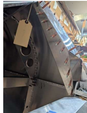
Updrilling LH former strap
