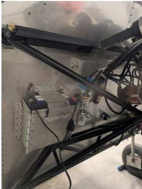
FWF electrical components mounted
