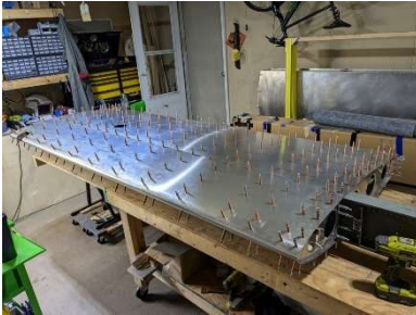
LH wing skin drilling complete
