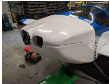
Upper cowl installed with spinner spacer
