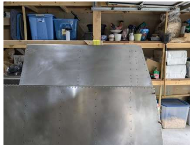
LH aileron installed (minus counterbalance)
