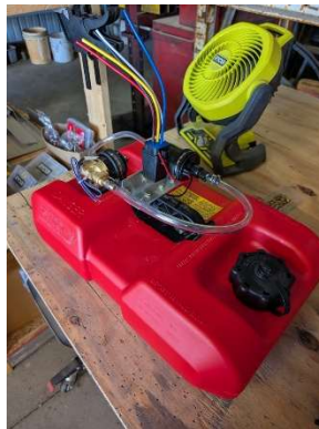
Smoke system components mounted to smoke tank
