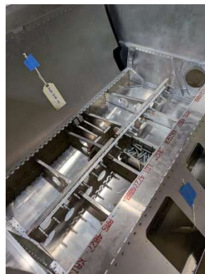
Hinges located and pilot drilled to forward seat pan channel
