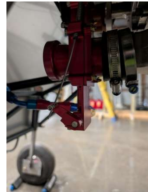
Mixture cable installed in AeroInjector. Idle cutoff position
