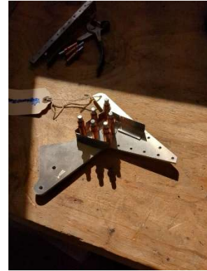
New rudder end cap clecoed
