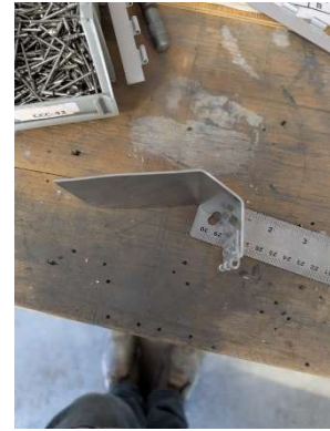
Battery box strap cut and bent
