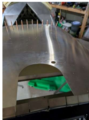
Hole cut in glareshield for fuel tank vent
