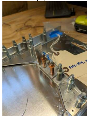
F14-12L located and pilot drilled
