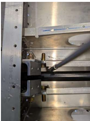
AN5 hardware installed in center seatbelt channel
