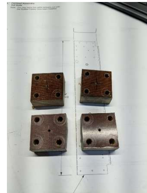
Rivet holes counterbored
