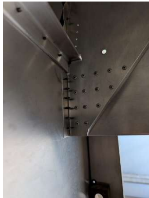
LH lower #1 former riveted to cross-tie box
