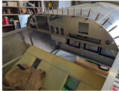
Panel cutouts complete
