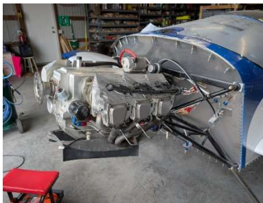
LH CHT and EGT sensors installed and wiring cleaned up
