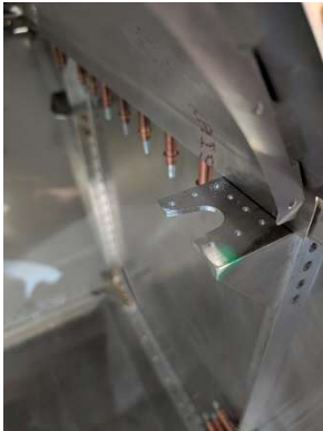
Corner plates updrilled
