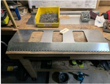
Forward seat pan assembly complete
