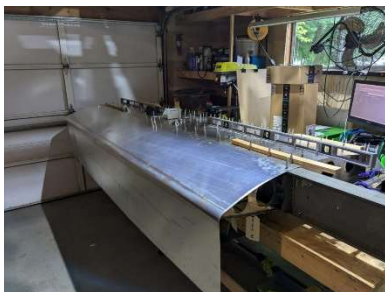
Starting to fit top side of forward wing skin
