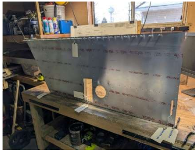
LH fuselage side panel pilot drilled
