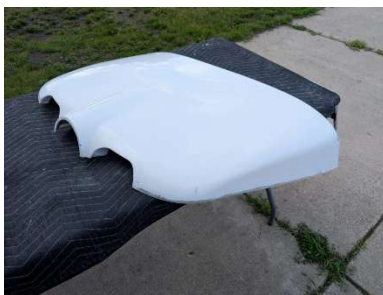
Finished sanding upper cowl
