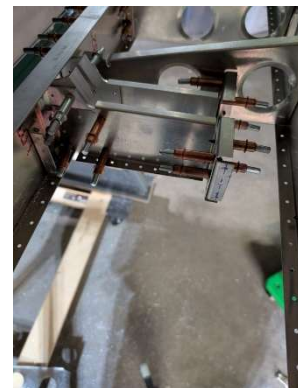
Removing ribs for better access to seat belt channels
