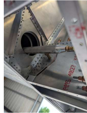
Updrilling rear wing attach angle to 1/2"
