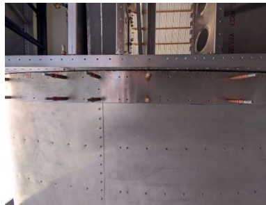
RH wing root doubler clecoed into place
