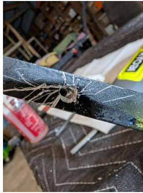
Tap removed and hole updrilled
