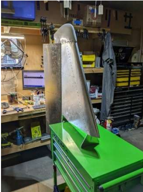
Completed vertical assembly
