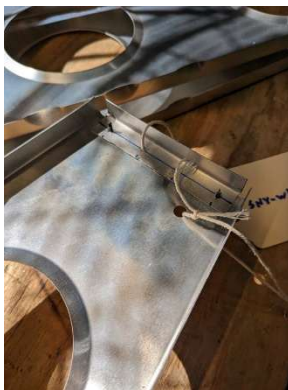
Aft tab added to #1 rib
