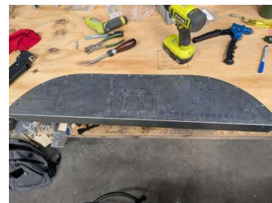
Center points drilled in circular voids
