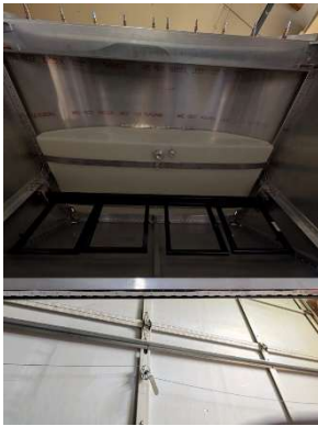
Fuel tank straps tightened
