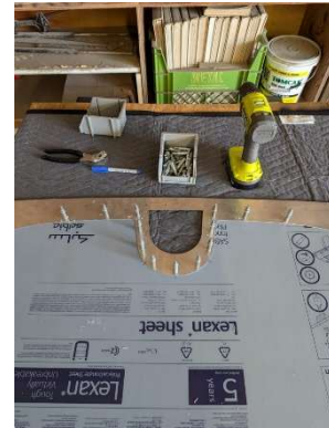
Pilot drilling fuel door holes
