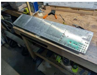
Aft spar tunnel web dimpled
