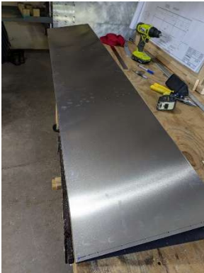
LH flap rib lines marked and pilot drilled
