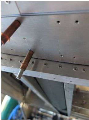
Spar bumpers riveted into place
