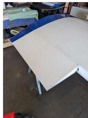
LH aileron installed with cotter pins
