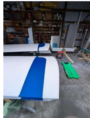
Wings taped, prepped, and partially masked
