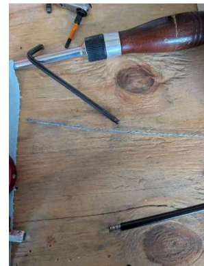
Throttle cable frayed and needs replacement
