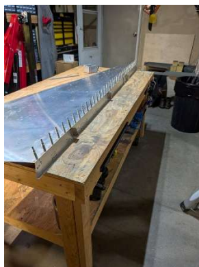
Locating and pilot drilling F20-07 splice channel to RH turtledeck skin
