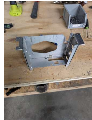
Side brackets installed onto GPS tray
