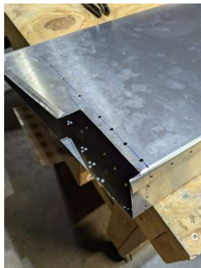
RH flap skin cut for pushrod clearance
