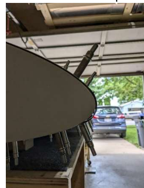
Slight gap in leading edge
