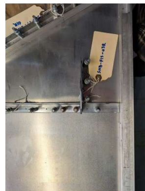
RH Rudder Pedal Mount Assembly located and pilot drilled
