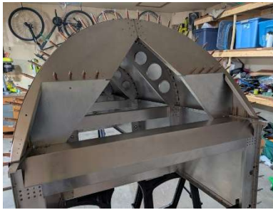
Upper/lower #1 formers fit and clecoed
