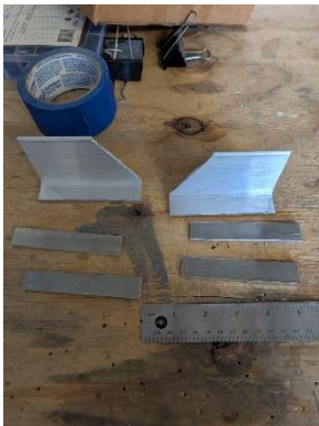
Master cylinder mount components cut
