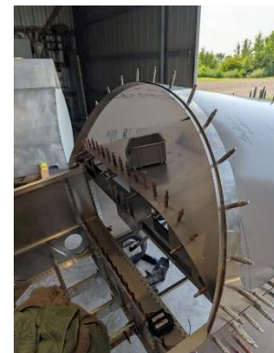
Bow strap pilot drilled to rear of windshield
