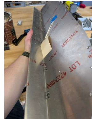
Bottom nutplates installed in panel blank
