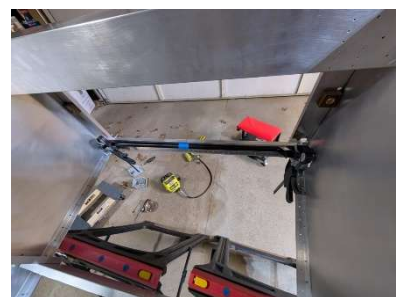
Drilling flap mount blocks to lower splice plates
