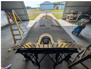
Bolts installed in forward part of windshield
