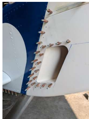
Side vents updrilled
