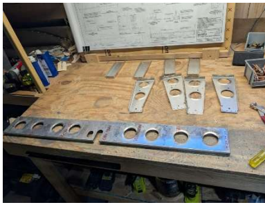
Seat pan ribs/channels deburred
