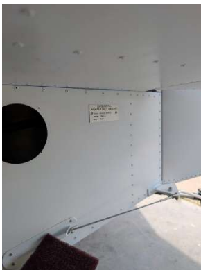
Data plate riveted to fuselage
