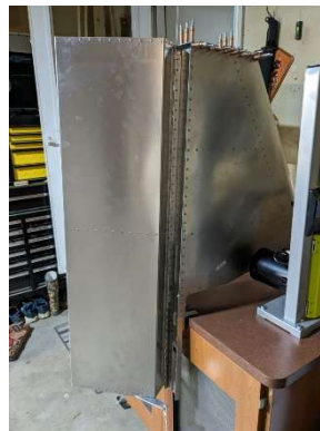
Noted rudder misalignment
