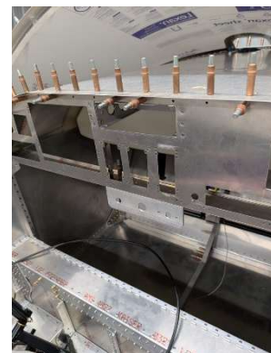
Lower panel angle clecoed into place
