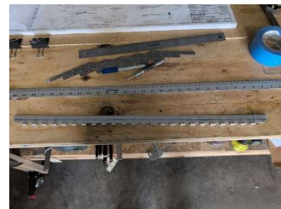
Canopy hinge cut and pilot drilled
