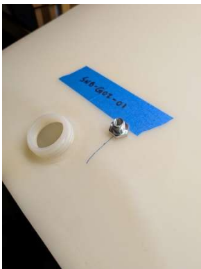
Installed fuel tank vent fitting
