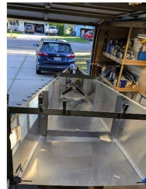
Setting uniform spacing throughout side panel assembly
