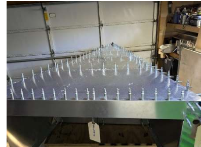
Aft fuselage floor pilot drilling complete
