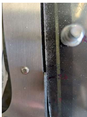
Checking clearance between canopy and fuselage
