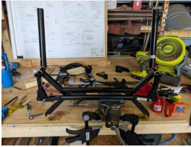
New control stick assembly nearly complete; just need to replace taper pins.
