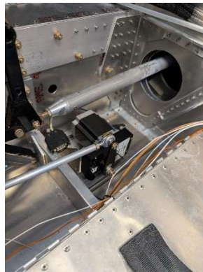
Roll servo installed and push rod connected
