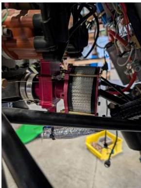
Air filter installed and AerolInjector safety wired
