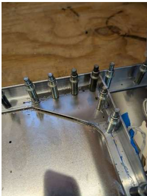
Seatbelt gusset located and pilot drilled
