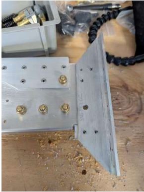
Rear spar holes updrilled to 1/4"
