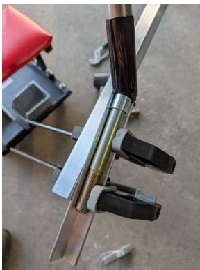
Axle toe in setup
