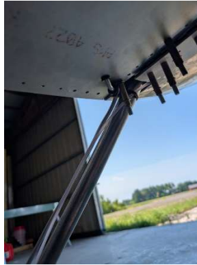
Fuel vent routed through floor and along LH gear leg
