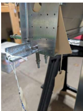
RH lower splice plate pilot drilled
