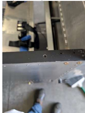
Alignment pin holes drilled in LH upper longeron
