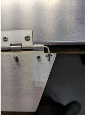
Trim tab safety wired
