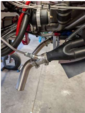
Air filter installed and AerolInjector safety wired
