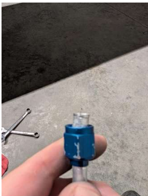
Improper flare on old fuel line
