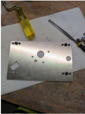
Nutplates installed for wheel Pant mounting
