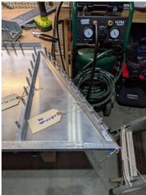
F14-01R assembly located and pilot drilled
