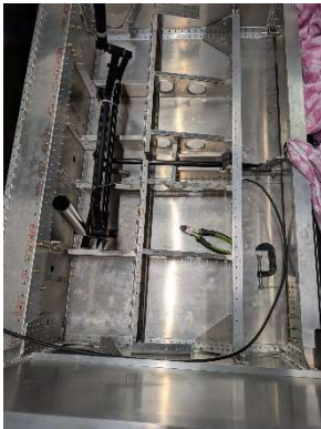
Trim cable routed through mid-fuselage
