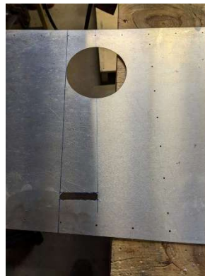
-01L rudder cable slot and inspection hole cut
