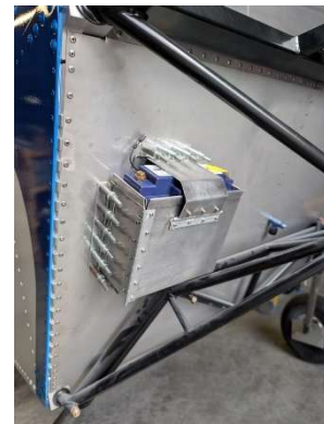
Battery box located and pilot drilled
