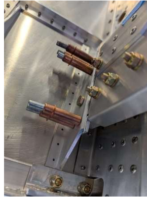
Locating RH rear spar attach angle onto fuselage side skin
