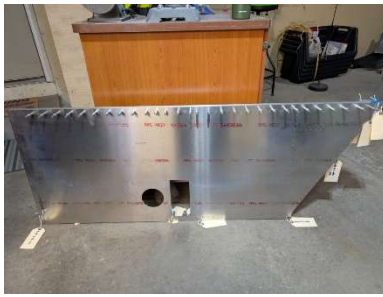
RH fuselage side panel pilot drilled
