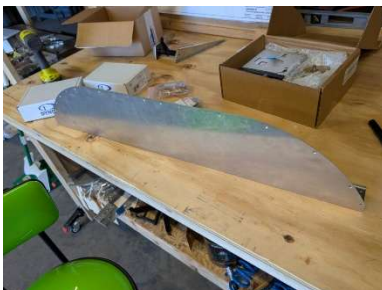
Some holes in panel dimpled for CCC flush rivets
