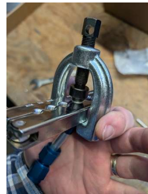
Flaring ends of hardline
