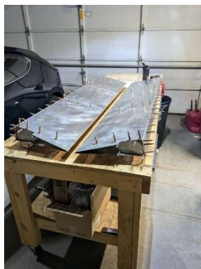
RH flap skin cut for pushrod clearance
