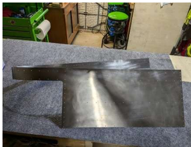
LH root doubler deburred and cleaned
