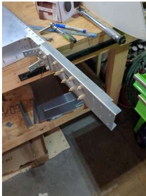
Vertical stabilizer rear spar
