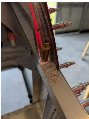
Windshield bow drilled to upper longerons
