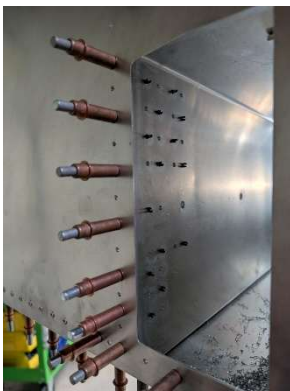
LH forward tunnel Zee updrilled
