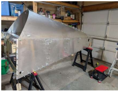
LH side of turtledeck skin located and partially pilot drilled/clecoed
