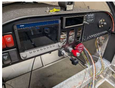
Trim wheel installed
