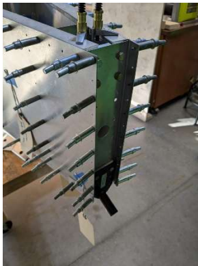
Aft fuselage channel pilot drilled and clecoed
