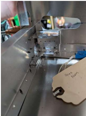
Holes drilled through spacers, lower splice plates, lower crossie, and aft fuselage floor
