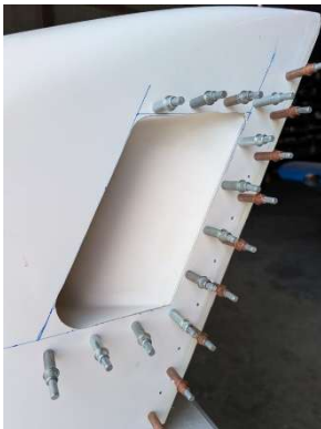
Pilot drilled and clecoed side exhaust vents
