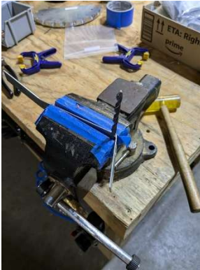
Bending -07 former clips with drill bit and vice
