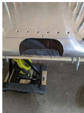
Skin dimpled for upper retaining angle
