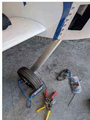
RH gear leg fairing installed
