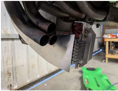
Oil cooler and baffling mounted
