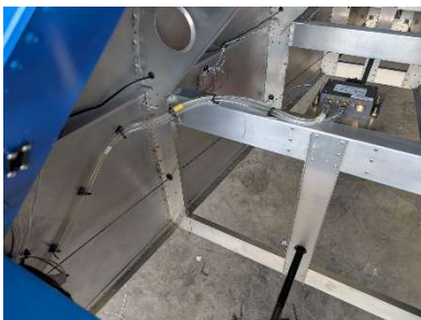
Pitot/AOA lines routed to ADAHRS box
