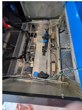
Fluid line routed through fuselage
