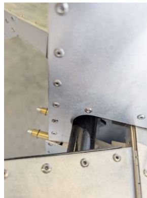
Interference between elevator horn and vertical stabilizer skin
