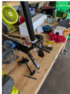
Hole ready to be reamed for taper pin
