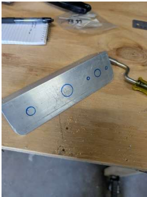
Holes marked in throttle support bracket
