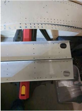
Root attach plates removed for conversion prep
