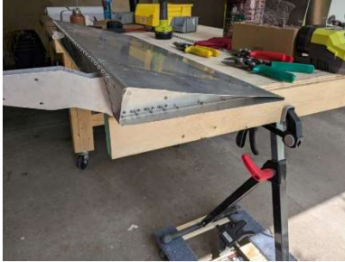
LH aileron skin trimming complete
