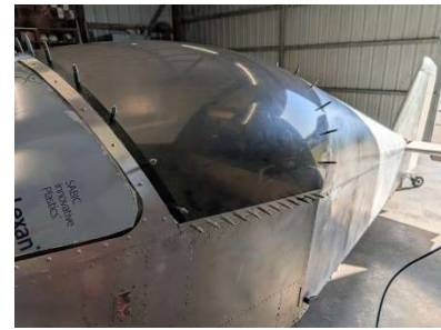
LH side trim clecoed into place
