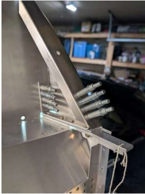
LH former clip pilot drilled
