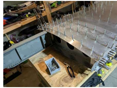
Aft root rib fitted
