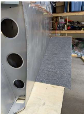
RH lower aft wing skin riveting complete
