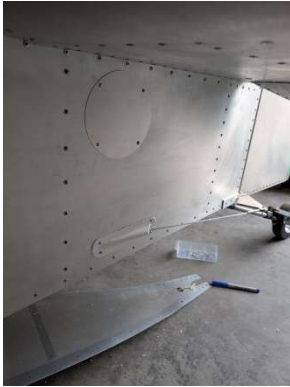
Cable fairings mounted onto fuselage
