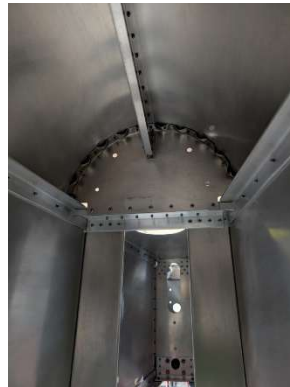
#5 former riveted to tail cone box
