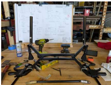
Bad stick assembly; control sticks not parallel to control horns
