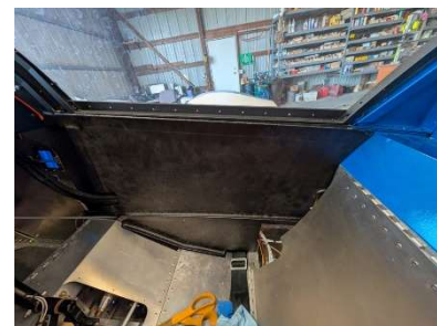
RH side panel installed
