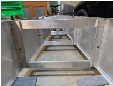
#2 upper cross tie riveted
