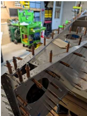
Aft shear web and tail angles updrilled
