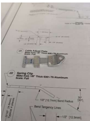
Aft spring clip cut and bent
