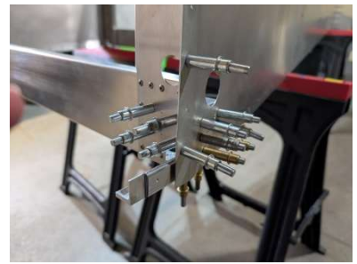
LH flap angle pilot drilled and clecoed
