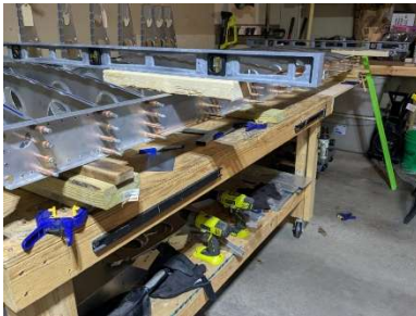
Rear spar locked into place
