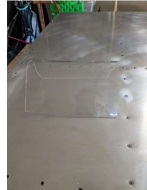
Landing light lens trimmed
