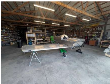
RH wing placed into spar box
