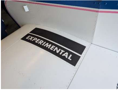
Wing walk grip tape and LH wing gap tape applied
