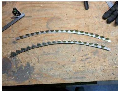
Firewall angles bent per plans (60-68 degrees)
