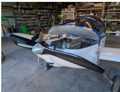
Prop reinstalled for test runs
