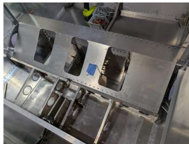
Forward seat pan installed with hinge pins
