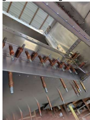
Rear spar carry through shear angle drilled
