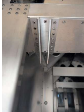
Flap motor mounts riveted per Revision E
