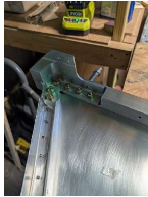
RH upper motor mount hardware installed
