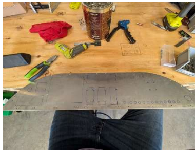
Bottom nutplates installed in panel blank
