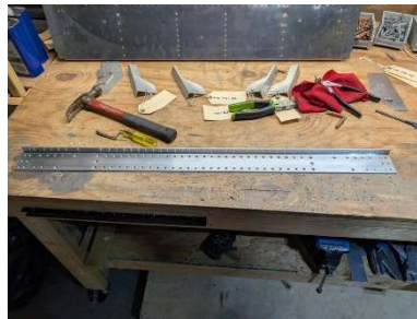
Support angle countersunk
