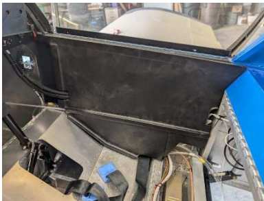
Rough fit of side panel to verify routing
