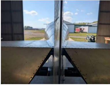
Fairing panels final fit
