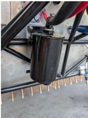
Oil separator moved up with new bracket
