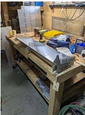
Rudder assembly pilot drilled
