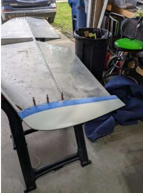
Installed LH tip
