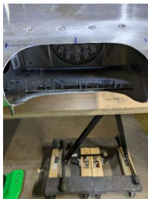
Holes drilled for upper lens retainer
