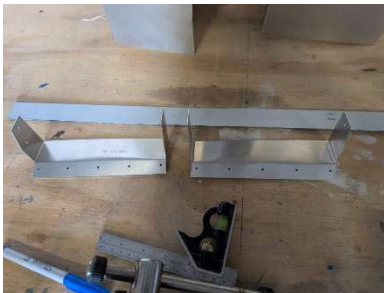
Exhaust outlet lips bent
