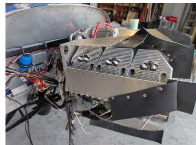
RH baffle access panel open
