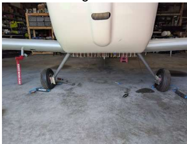
Gear leg fairings installed on gear legs
