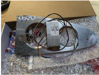
Pitot controller installed on #4 forward rib
