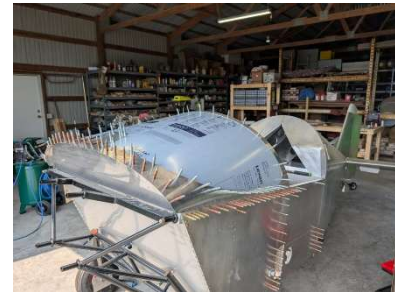
LH side longeron holes updrilled
