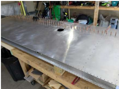
LH bottom side wing riveting in progress
