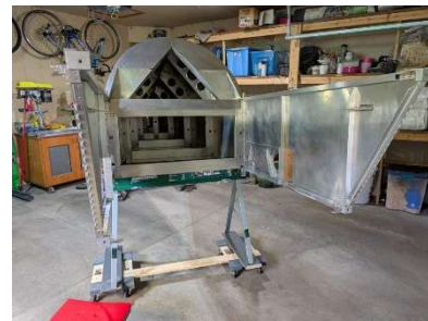
Forward side panels clecoed into place
