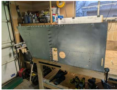
Bolts installed and torqued
