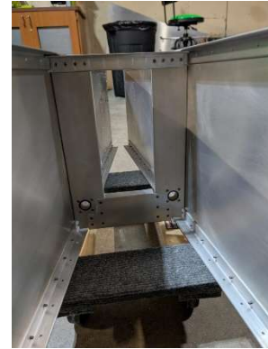
Aft angle and crosstie #5 riveted
