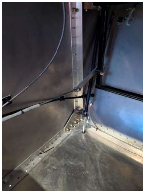
Fluid line routing through firewall
