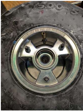
Torqued wheel bolts and setting bead
