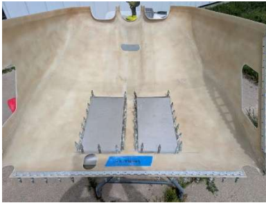
Exhaust tunnels clecoed to lower cowl
