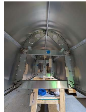
Aft fuselage station #3 updrilled
