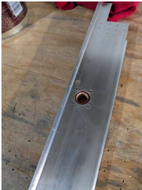
Cable fairlead blocks riveted
