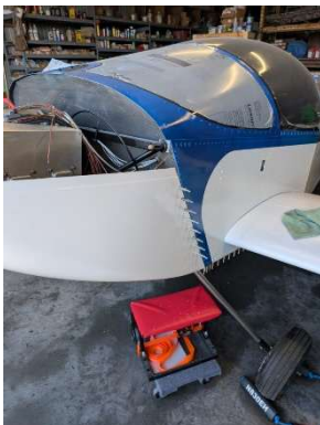
Side hinges pilot drilled to cowl
