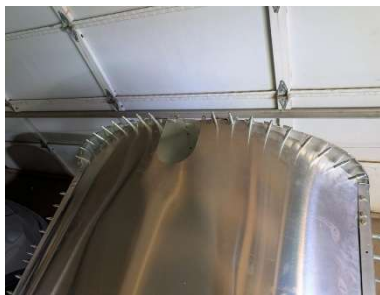
Forward edge of glare shield pilot drilled
