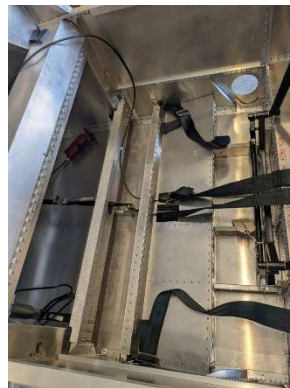
Aft seat pan riveted
