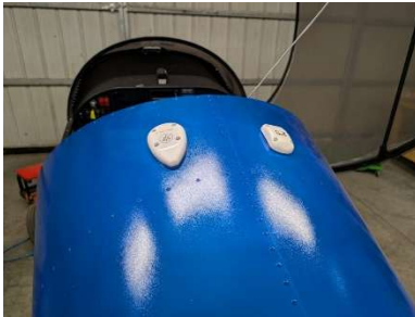
Both GPS antennas mounted
