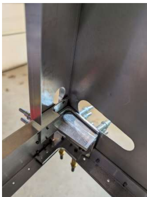
Lower crosstie notched for flap mount blocks
