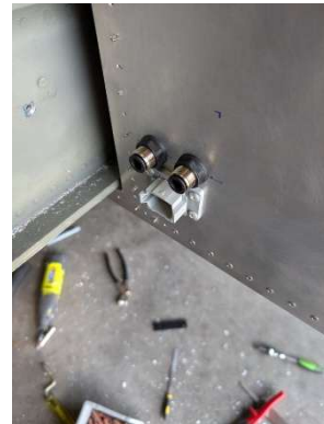
Pitot and AOA tube connectors mounted
