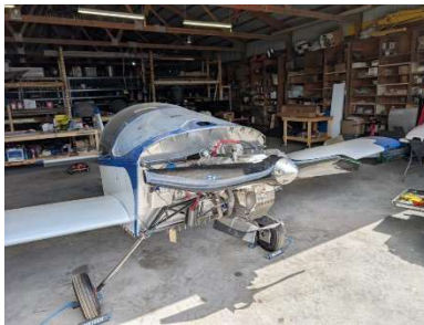
Prop and spinner installed
