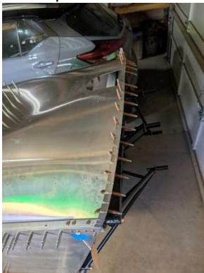
Firewall and glare shield updrilled
