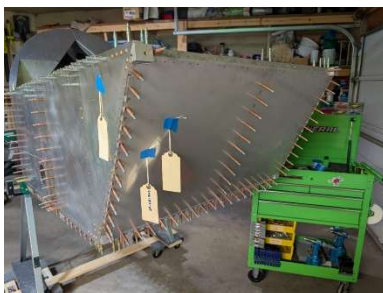
Lower firewall updrilled
