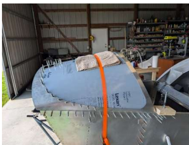
Pilot drilling continued and strap added to help curvature of assembly. Note blocks on upper longerons to hold windshield forward.
