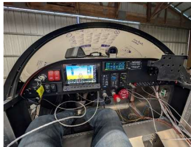
Intercom installed and ops check good
