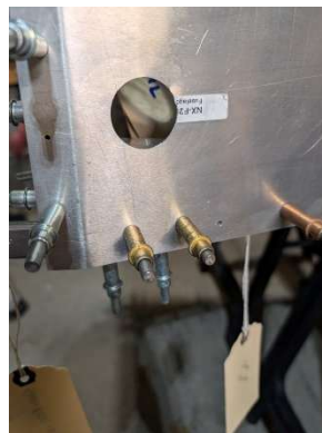
LH bolt holes through lower splice plate
