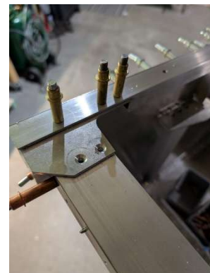
Upper forward cross tie updrilled and countersunk
