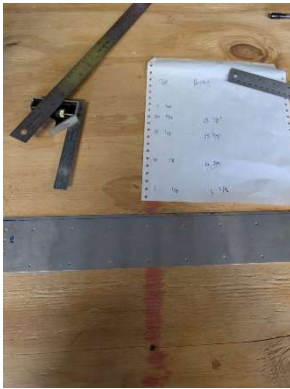
Marking trim line from measurements on wing skins
