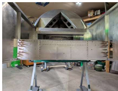
Aft spar tunnel web clecoed to fuselage
