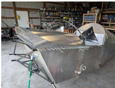
Windshield skirt installed and clecoed to upper longerons
