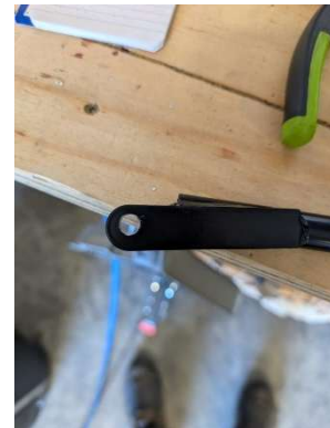
New hole drilled in LH side of link rod
