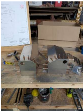
Baffles updrilled and clecoed
