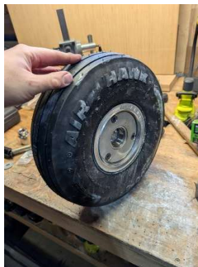
Wheel halves assembled and brake disk installed with new bolts
