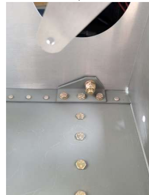
LH tie down bolt torqued
