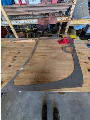
Marking overlap lines on windshield skirt
