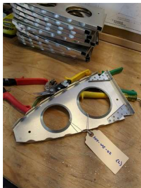
Forward rib with gussets attached
