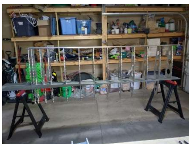
LH wing rib installation complete
