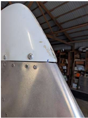
Marking how much fill needs to be added to fairing tip
