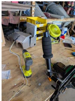
Foam grip installed and holes drilled. Using safety wire to thread control wires through opening
