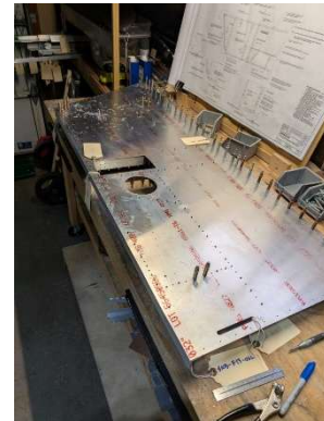
Updrilling bolt holes
