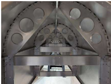
Formers #4 through #2 clecoed into place
