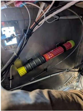
Fire extinguisher mounted on forward fuselage side panel
