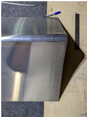
Trim line laid out
