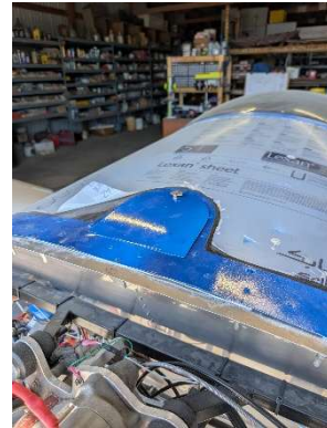
Fuel door installed
