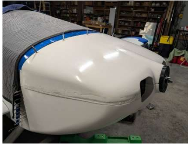
Upper cowl screw holes pilot drilled and attached to upper cowl shelf
