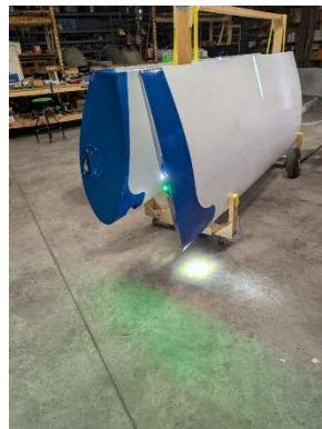
Testing RH wing lights
