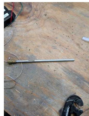
Fuel probe trimmed
