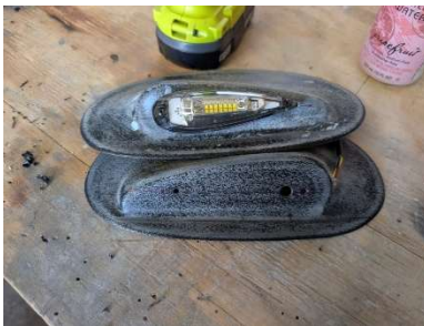
Tip light mounting holes drilled in fairings
