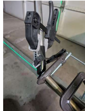
V Block used to pilot drill gear legs and axles
