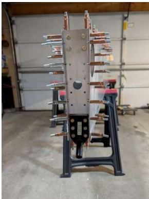
Tail channel fit and bolted into place
