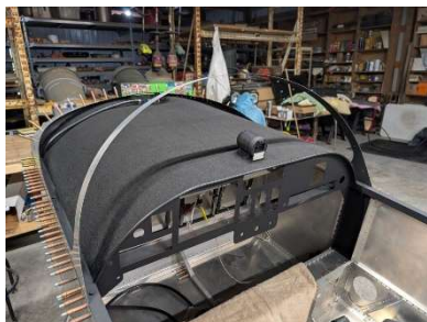
Windshield skirt clecoed into place
