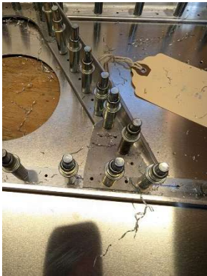
LH upper gear gusset located and pilot drilled
