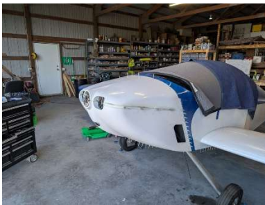
Upper and lower cowls pilot drilled
