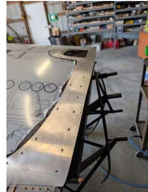
Upper firewall riveted to windshield skirt
