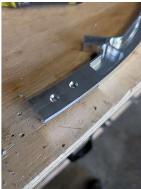
Countersinking rivet holes for flush rivets
