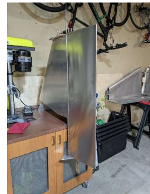
Noted rudder misalignment
