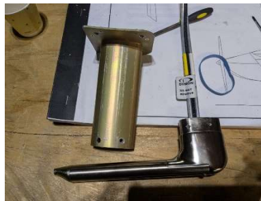
Holes upsized in mount mast
