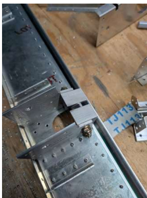
Seat belt mounts bolted
