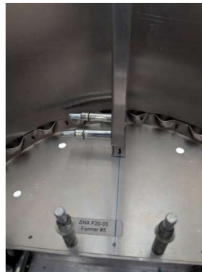
Aft clip located and pilot drilled to skin splice channel and former #5
