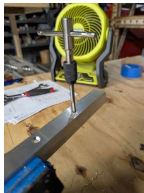
Taping outside holes for canopy alignment pins
