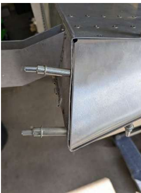
.032" spacer installed in RH aileron tip rib
