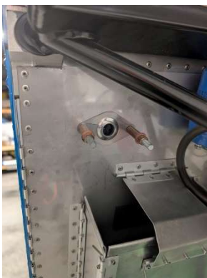
Grommet plates clecoed into place
