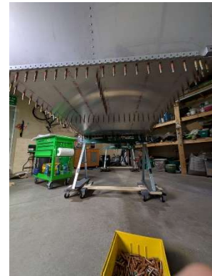
Forward fuselage floor clecoed into place
