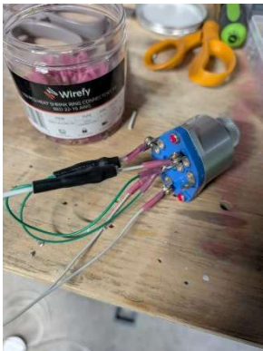
Switch end of ignition harness complete
