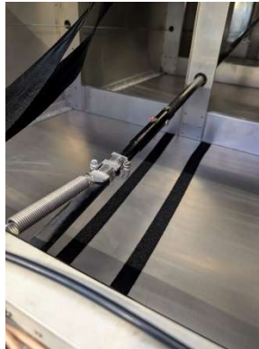
Velcro strips applied to baggage compartment floor
