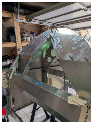
Former #1 assembly clecoed into place
