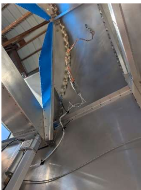
Dynon GPS antenna run (will clean up later)
