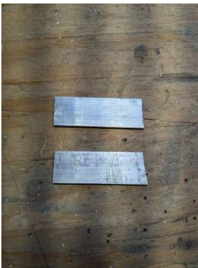
-08 rudder stops cut
