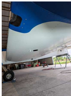
LH under wing color sanded and buffed
