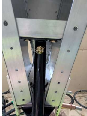
Tail wheel spring hardware installed. Shimmed length with washer each side of mount tube.
