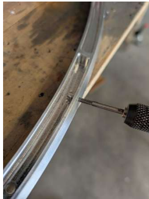
Tapping bow holes for 6-32 screws
