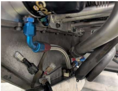
Oil cooler hose #1 installed
