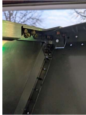
Hardware installed in LH upper motor mount
