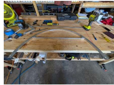
Aft canopy bow cross tube installed
