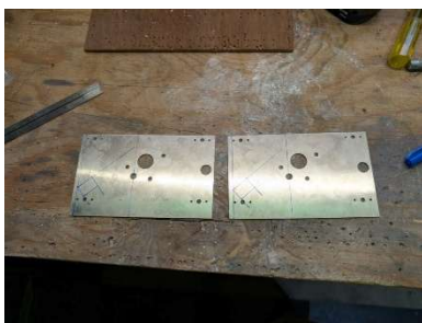
Marking wheel pant mount plates
