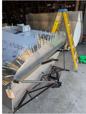
Windshield skirt clecoed to upper firewall
