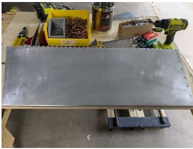
LH aileron scotchbried and cleaned
