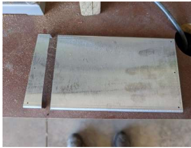
Dynon-supplied stiffener trimmed
