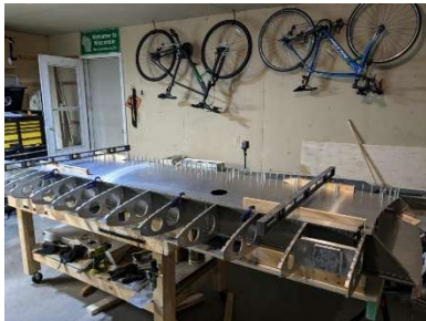
RH aft lower skin in progress
