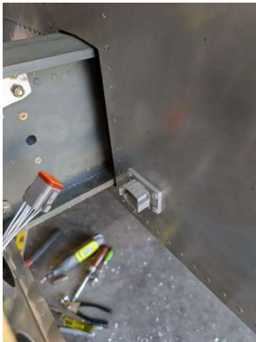
Slid out RH wing and located bulkhead connector
