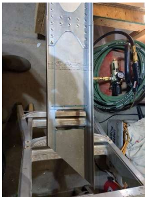
Cutout for aileron counterweight
