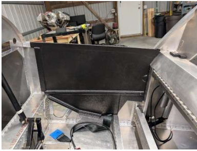
Testing fit of fuselage side panel
