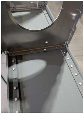
#5 aft rib installed
