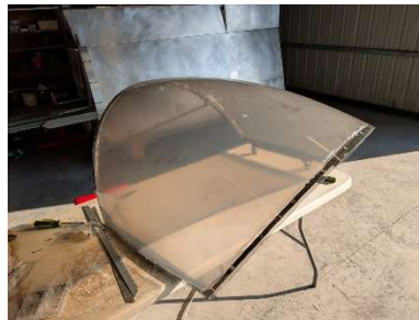
Canopy being attached to frame
