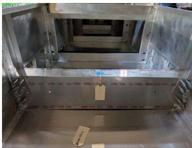
Forward tunnel z located and pilot drilled
