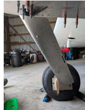
RH fairing installed
