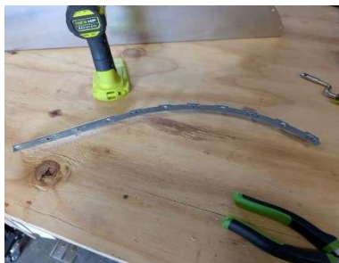
Nutplates installed in right panel flange
