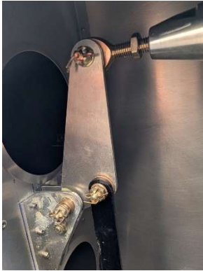
RH aileron pushrod installed onto bell crank
