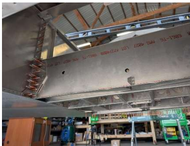
Forward tunnel zee reinstalled
