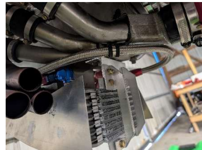
Oil cooler hose #2 installed
