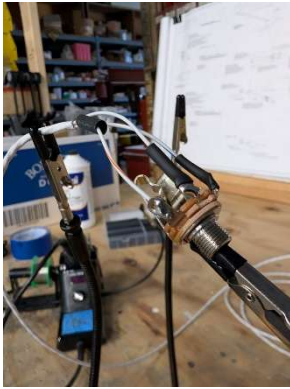
Copilot headset jack soldered
