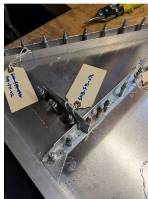
LH rudder Pedal mount assembly pilot drilled
