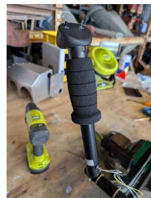
Stick grip secured with set screw
