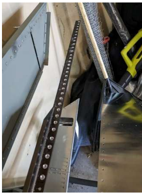
LH upper spar cap countersunk
