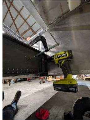
Drilling rear wing attach angle using drill guide
