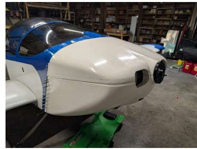
Marking fiberglass overlap line
