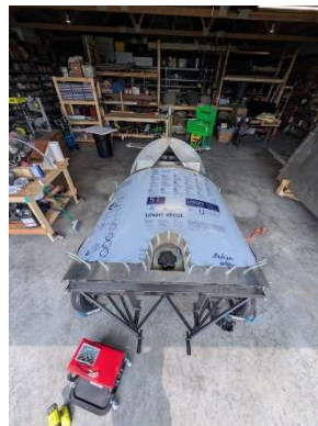
Windshield inserted and starting to drill to skirt
