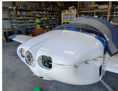
Mounting holes updrilled
