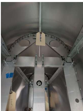
#4 formers clecoed and pilot drilled to turtledeck skin
