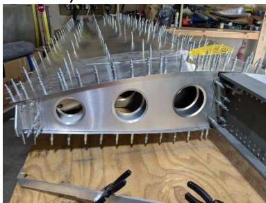
LH aft root Rib pilot drilled
