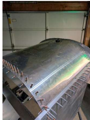
Fuel tank stop riveted to glareshield
