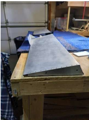
Checking twist in control surface
