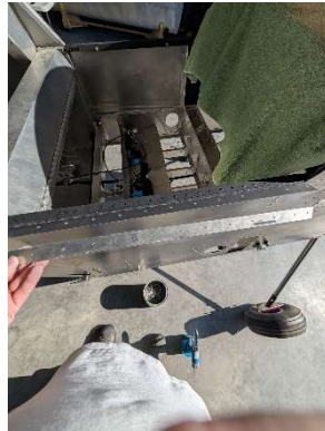
Hinge and trim holes updrilled
