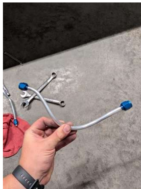
New fuel line cut and bent
