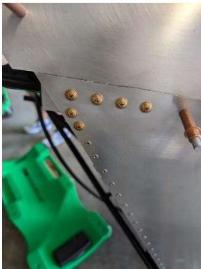
Upper motor mount bolts installed
