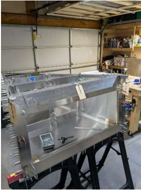
Cross Tie installed on aft tail cone
