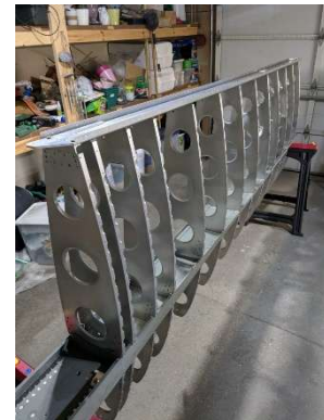
LH wing rib installation complete
