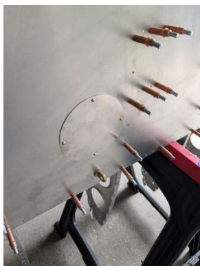
Aileron bellcrank inspection plate installed
