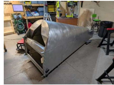
Aft fuselage floor clecoed into place. F18 complete!
