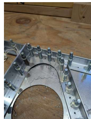
LH lower gear gusset located and pilot drilled
