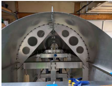
#2 formers clecoed and pilot drilled to turtledeck skin
