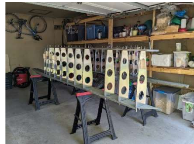
Aft rib mockup on spars Aft rib mockup on spars
