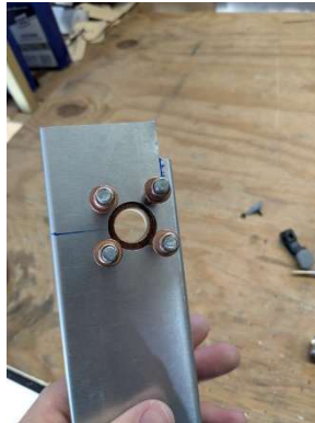
Fairlead mount block clecoed in place
