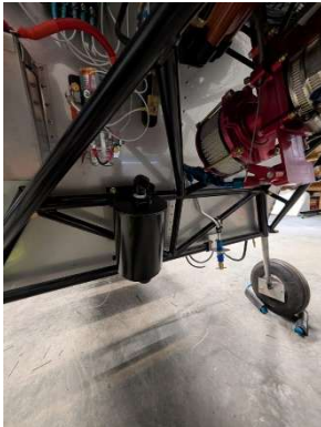
Oil separator mounted
