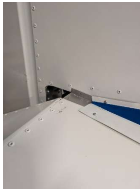
Test fitting of fairing angles
