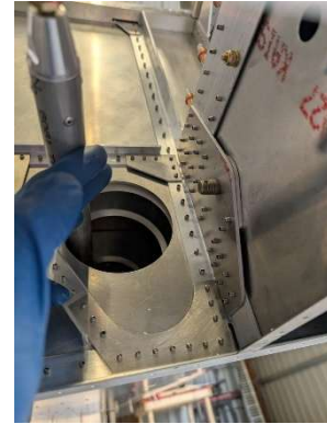
LH main wing attach angle drilled
