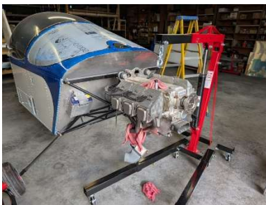
Placing engine using engine hoist
