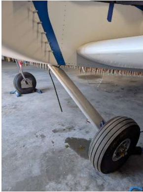
LH gear fairing fitted to landing gear
