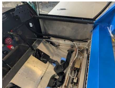
RH cable bundles and pitot/AOA tubes secured to RH fuselage side
