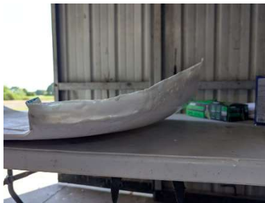
Micro mixture applied to outside lip of cowl
