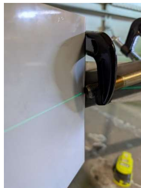
Axle height set via laser level
