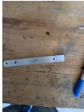
LH cable adjuster hole drilled and trim line marked
