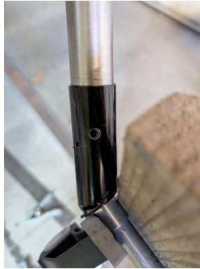
RH axle hole misaligned
