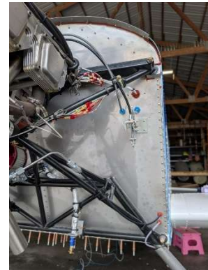
Firewall sealant on LH side
