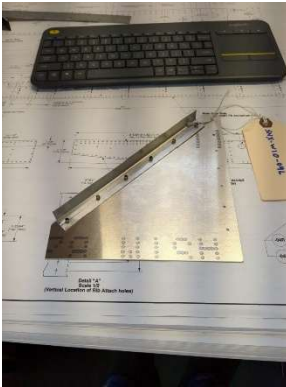
Inspection of wing tip rib
