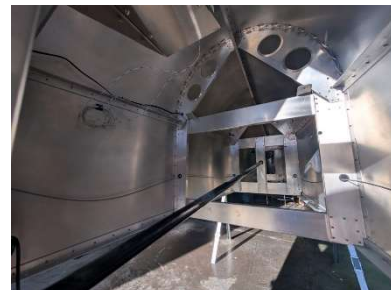
OAT probe and ELT remote wires run from tail section
