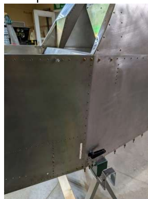
LH side panel riveted and hardware installed
