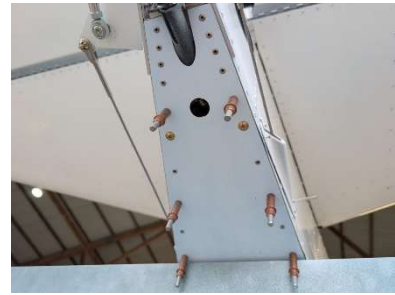
Tailwheel mount bulkhead bolts installed
