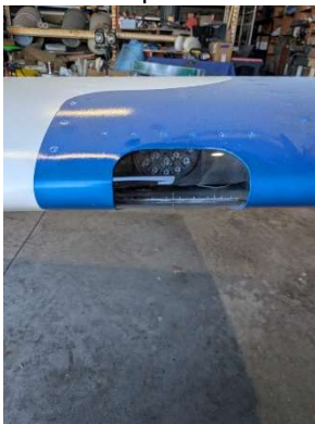
LH landing light lens installed
