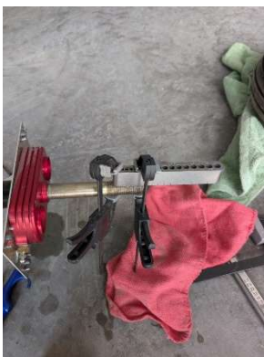
Used drill guide to drill cotter pin holes
