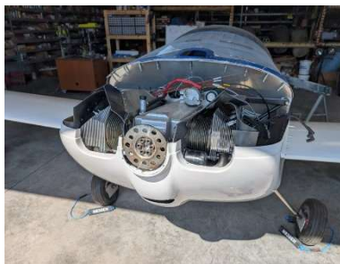
Test fitting cylinder baffles
