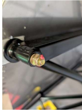
Marker paint added to bolts
