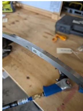
Installing flush solid rivets into canopy bows
