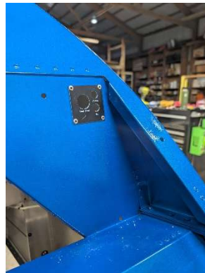
Headset panels installed
