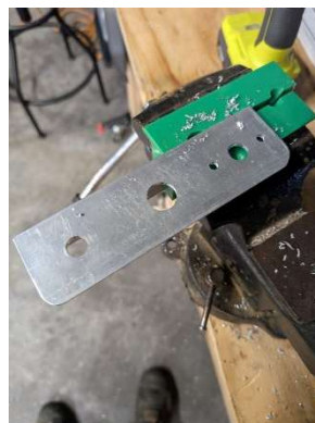
Lower panel holes drilled
