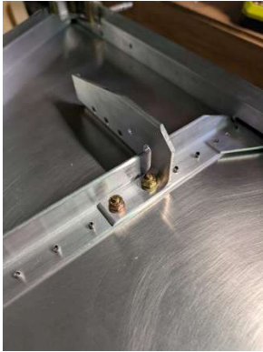
RH rudder pedal mount assembly bolts installed
