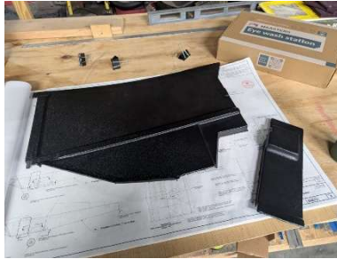
Trimmed RH side panels. Still need to be cleaned up
