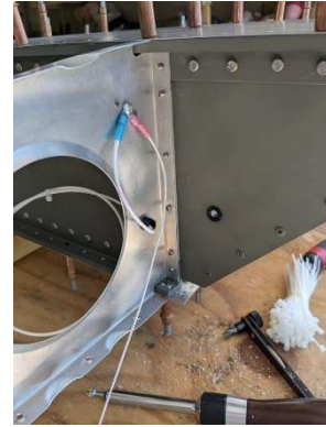
Bushing installed in tip web
