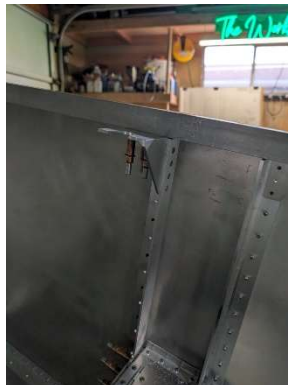
RH panel mount riveted
