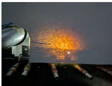
Used flashlight method to locate lower cowl hinge holes
