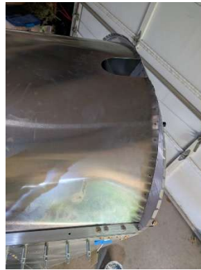
Glareshield riveted to firewall angles
