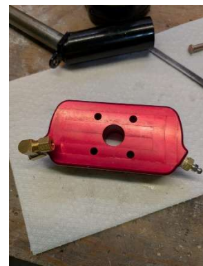
Fittings attached to brake body using Teflon paste
