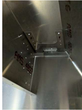
Underneath view of cross tie box
