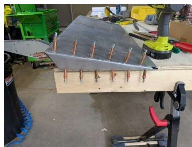
LH aileron tip rib clecoed in place
