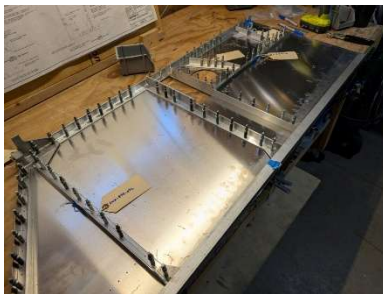
F15-10 gussets pilot drilled
