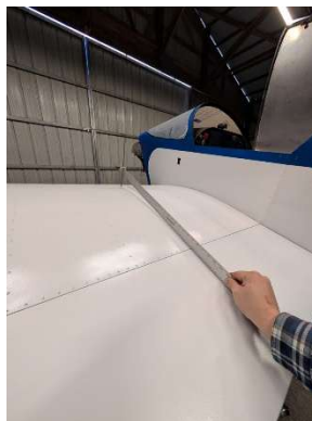
Checking LH flap neutral position
