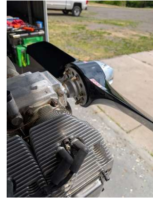
Prop and spinner bolted to engine
