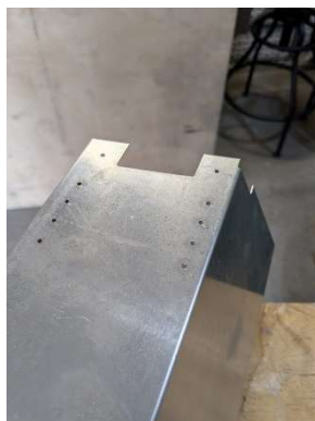
Extra holes in cross tie box drilled
