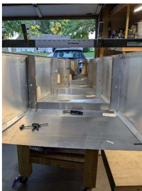
Bottom cross ties pilot drilled
