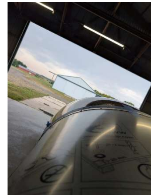
Canopy slightly bulging on sides
