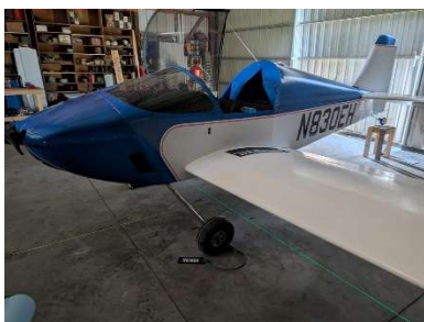
Using tape measure and laser level to determine equipment arms
