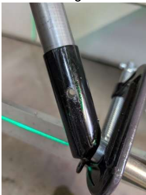
Axle drilling complete!
