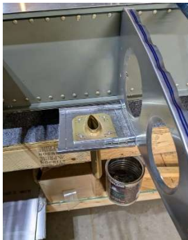
Skin doubler for pitot mast mounted
