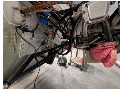
Oil separator line installed
