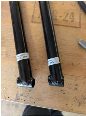
Pilot holes drilled in stick grips
