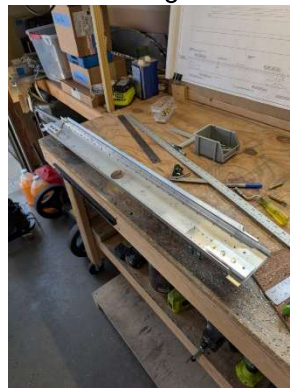
Rear spar carry through clecoed together
