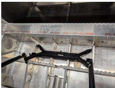
Temporarily installed stick frame
