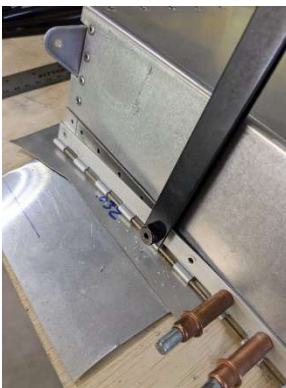
Redrilling hinge half with strap duplicator
