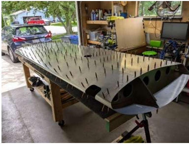
RH bottom wing skins updrilled
