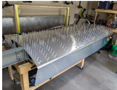
LH forward wing skin pilot drilling complete on top side
