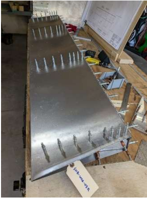
RH flap lower side pilot drilled
