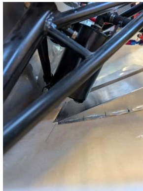
Oil separator now clears exhaust tunnel
