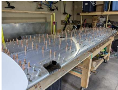
LH underwing updrilling in progress
