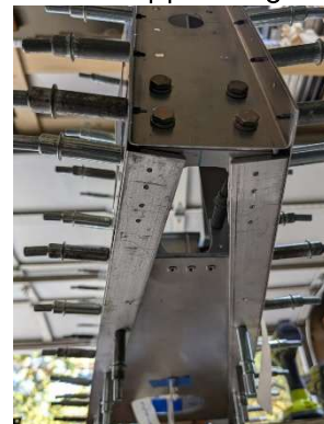
Holes drilled through aft lower mount angle and lower longerons
