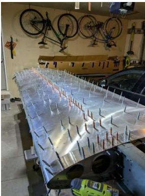
Updrilling in progress
