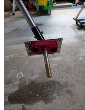
LH brake assembly mounted
