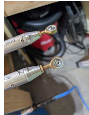
Rod end bearings installed
