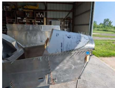
Forward and side windshield holes pilot drilled
