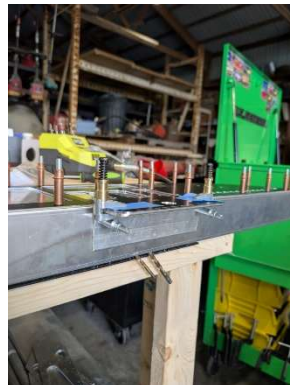
Throttle support angle located and pilot drilled
