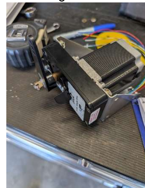
Roll servo installed into bracket and limiter installed
