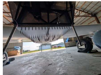
Forward fuselage floor clecoed
