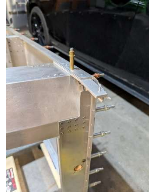
Cross tie box riveted to #1 vertical channel and cross tie box splice plate
