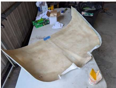
Micro mixture applied to inside edge
