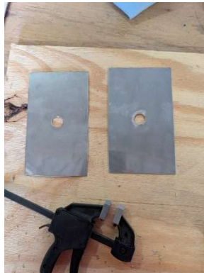
Mount plates cut and drilled out of stainless steel
