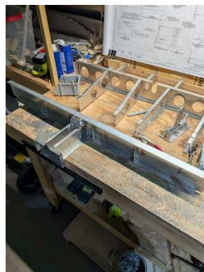
Idler assembly riveted to seat belt mount assembly
