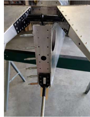
Temporary spacers removed from tail channel
