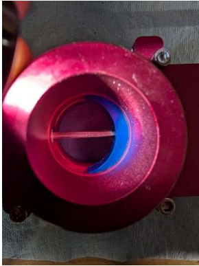
AerolInjector reassembled and 2.5 needle installed
