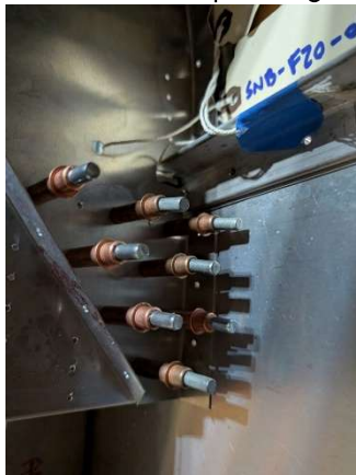
RH lower Former updrilled
