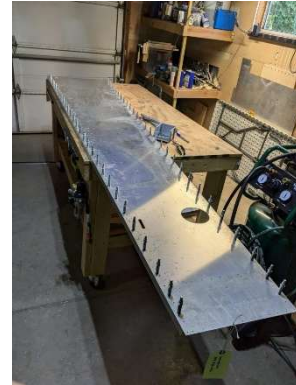
LH lower longeron pilot drilled in place and offset for bottom skin
