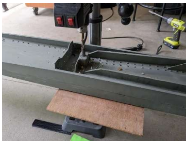
Drilling 3/8" hole with guide
