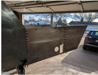
RH forward side panel clecoed into place
