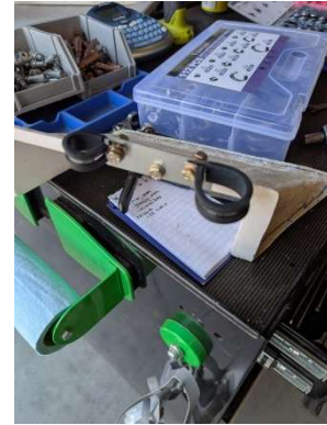
Preheat and battery charger cord mount in cowl exhaust scoop
