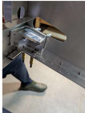
RH flap angle pilot drilled and clecoed
