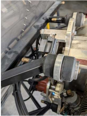
Engine mount detail with temporary washers
