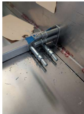
Aft floor angle pilot drilled
