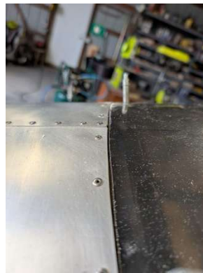
Working on preserving 1/16" gap on aft side of canopy
