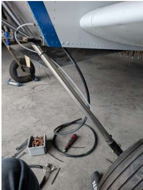
Brake lines routed to calipers
