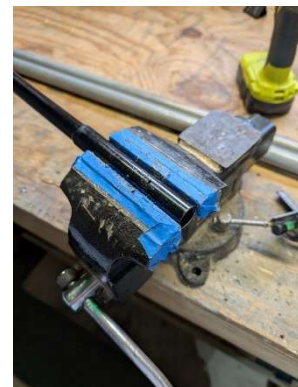
Pilot drilling holes for -05 elevator pushrod end
