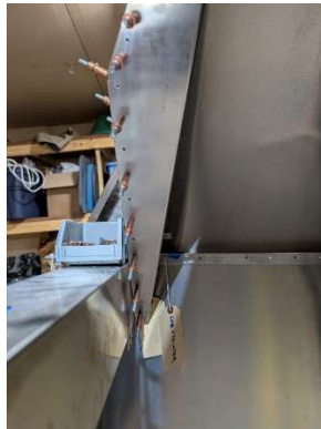
Updrilling RH former strap
