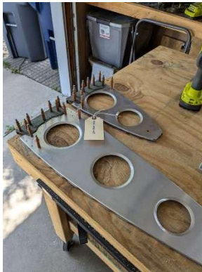
Root ribs updrilled
