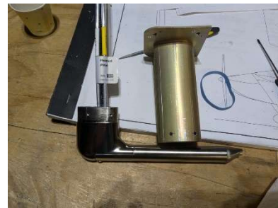
Holes upsized in mount mast
