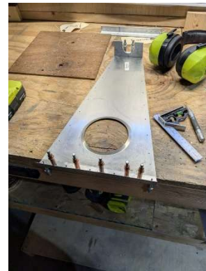
Assembly of -02 aft shear plate
