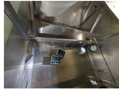
Aft tunnel web located and clecoed
