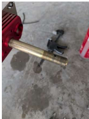
Cotter pin holes drilled
