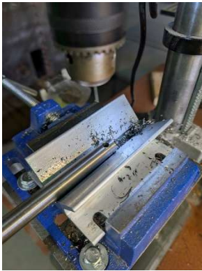
Updrilling tail wheel spring with drill press
