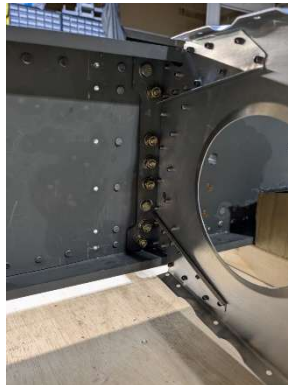
LH aft root rib installed
