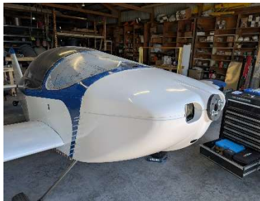
Trimming of upper cowl continued
