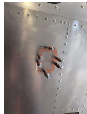
Drilling doubler holes and marking vent cutout
