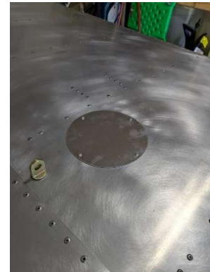
LH aileron bellcrank inspection cover installed
