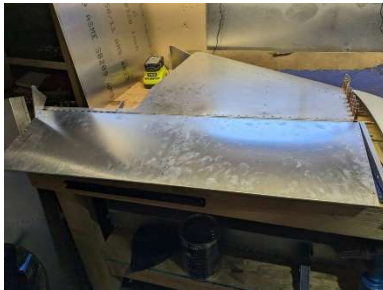
Hinge rivets finished
