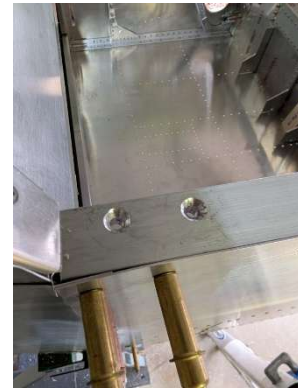
RH upper longeron countersunk for flush hardware
