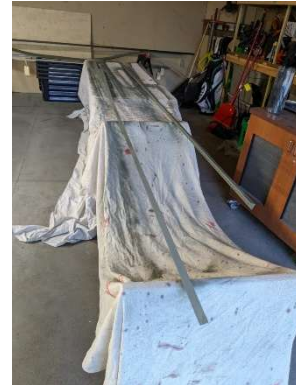
Priming the RH main spar parts
