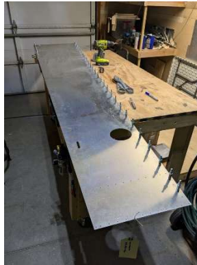
LH upper longeron pilot drilled in place
