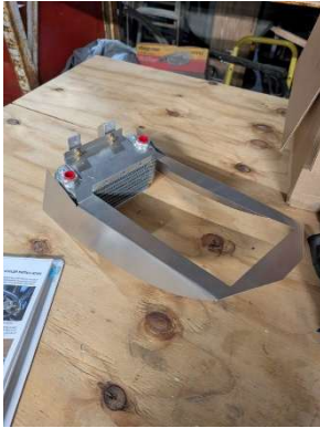
Oil cooler baffling installed
