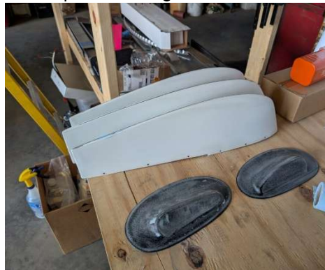
Fiberglass ready for paint
