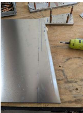
Drive plate underside notch- out laid out
