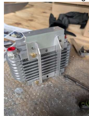
Oil cooler brackets installed
