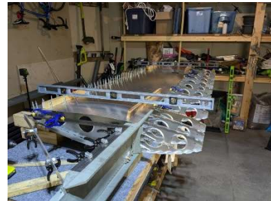
Inboard section leveled
