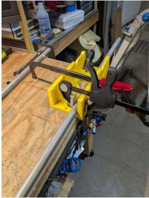
Cutting aluminum pushrod tubing
