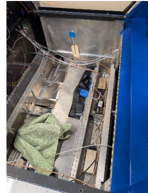
Routing transponder and ADS- B harnesses
