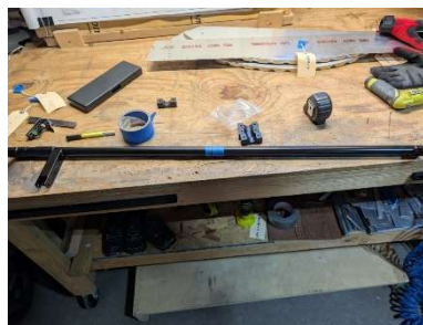
Flap drive tube center marked
