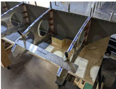
Mounting plate nutplates installed
