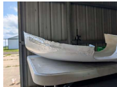
Micro mixture applied to outside lip of cowl
