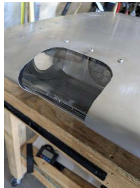
Landing light lens installed
