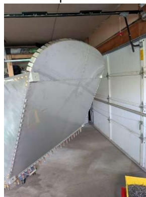
Upper firewall riveted
