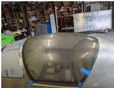
More trimming and began clecoing canopy to frame
