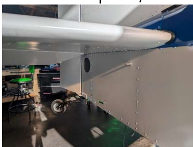
OAT probe installed under tail
