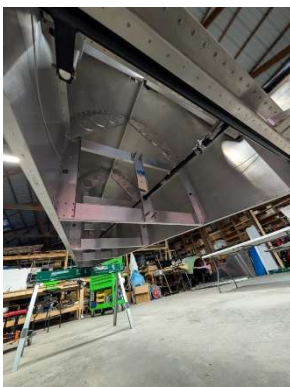
Aft fuselage floor removed
