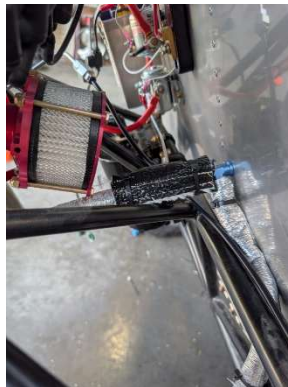
Fuel pump insulated
