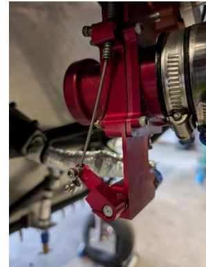
Mixture cable installed
