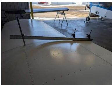
Neutral position set with ruler and straight edge
