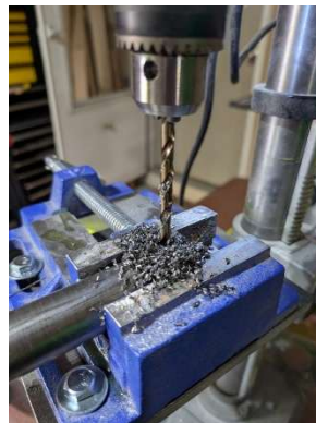
Updrilling main gear leg attach hole
