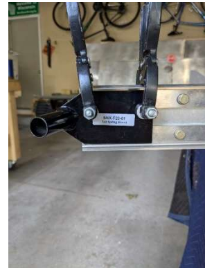
Tail wheel mount clamped into place on vertical stabilizer
