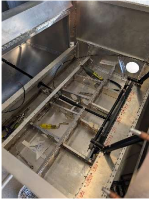
Elevator assembly temp installed
