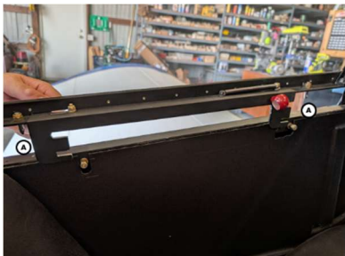
Step 1: Guide the canopy alignment pins (A) into the corresponding holes in the upper longeron.
