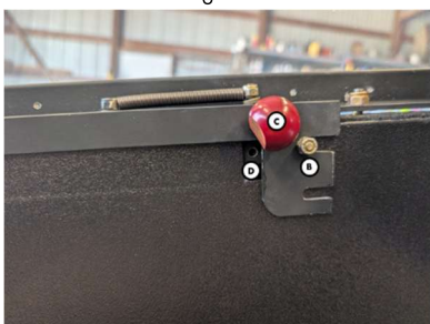
Step 3: Push the canopy latch handle (C) fully forward so the slot in the latch engages the latching posts (B). The canopy is fully latched when the lock pin hole (D) is fully visible.
