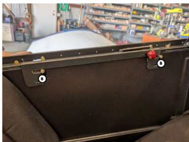
Step 2: Align the top slots in the canopy latch with the latch posts on the cockpit side rail (B)
